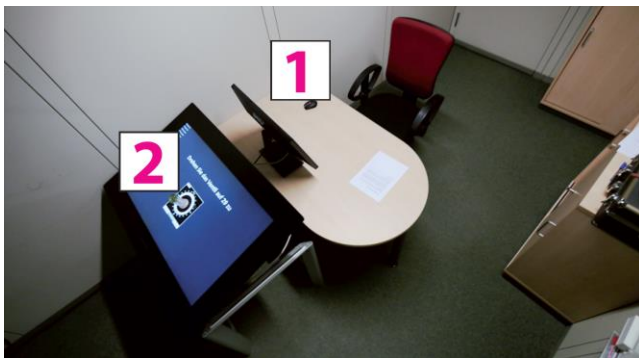
Figure 7. Traditional interaction styles at a desktop system (1) and post-WIMP interaction at a Samsung SUR40 (2); both with a resolution of 1920 x 1080.
