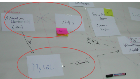
Figure 3: The evolution of the concept map, including an additional MySQL database. The changes are made explicit by crossing out earlier links between the data source and the db4o and introducing a link back from the visualization to the db4o.
