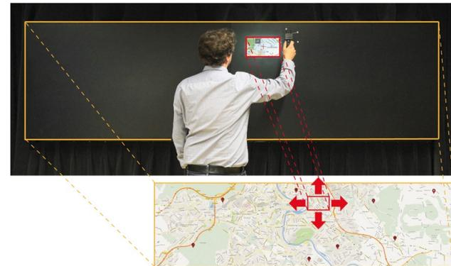
Figure 3. Map navigation using a (simulated) tablet sized peephole [12].
