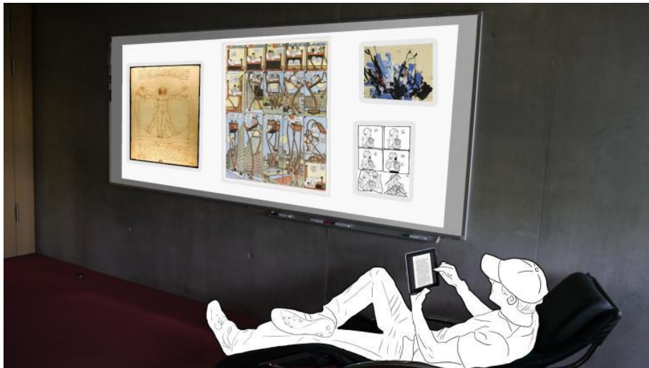
Fig. 1. This sketch illustrates the idea of the “ Interactive Reading ”. It supplies the user with additional information on a secondary wall-sized display while reading a document on an e-book device.
