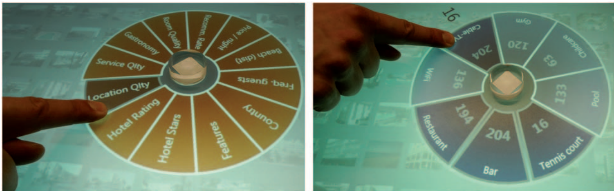
Figure 2. Assigning the desired data field (left) and value range (right) to a query token using touch input.
