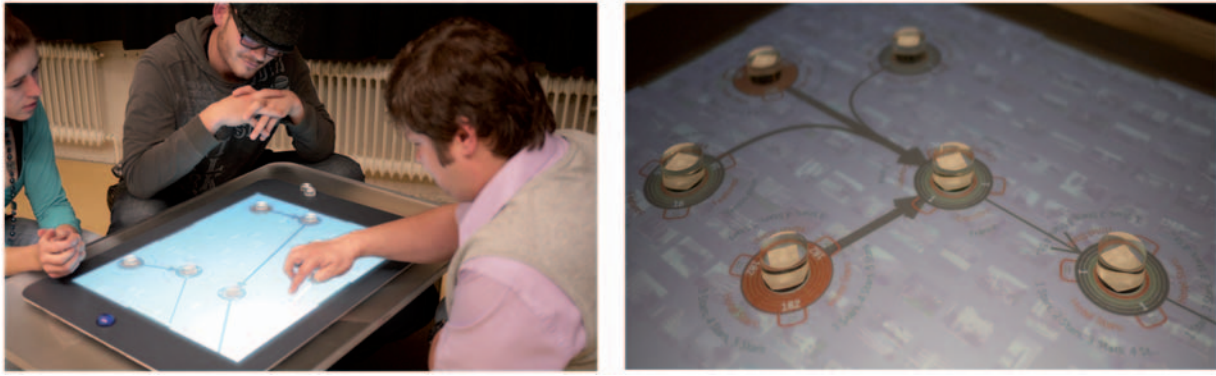
Figure 1. The Facet-Streams system for co-located collaborative search on tabletops (left). Glass tokens form a tangible filter/flow representation of faceted Boolean search (right).
