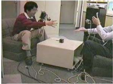
Figure 1. "Transvision" [7], a design tool where collaborators look on a real table-top through a palmtop-sized see-through display. 3D data from the display is processed by an external graphics workstation.
