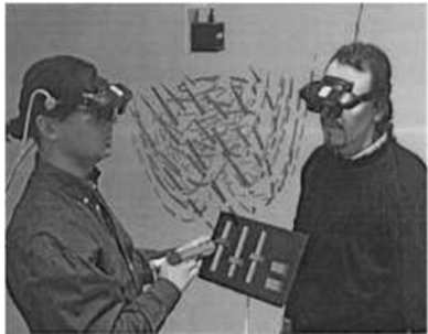
Figure 2. "Studierstube" [8], a system capable to visualize three-dimensional, scientific data with see-through glasses. Tracking data is processed on an external tracking server.
