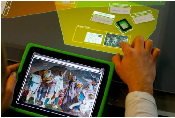
Figure 6. Tapping a result in the result view (shared display) triggers the result view on the private display.
