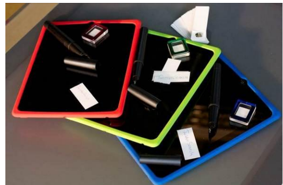
Figure 2. Three TwisterSearch sets, each consisting of an Apple iPad, an Anoto pen, a token, and several paper snippets.
