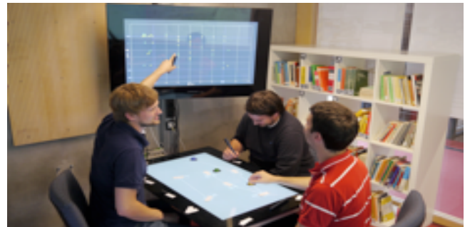
Figure 1: The setting of the VIS system consists of a horizontal display for query formulation and a vertical display for data exploration. Digital pen and paper is used for keyword input.
