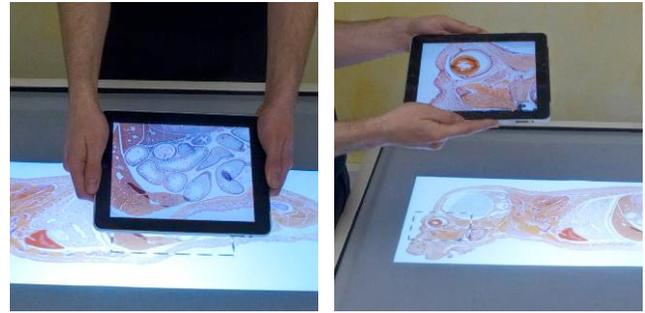
**Figure 2. The iPad is used to explore a high-resolution image of a cut through a rat. Lowering and lifting the device controls the zoom factor, whereas horizontal movements allow for panning. Due to the marker less tracking provided by the Kinect, no markers need to be attached to the iPad.**
