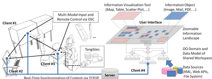
**Fig. 1.** A ZOIL-based multi-user, multi-surface, and multi-device interactive space (left). The right section shows the architecture and user interface of a ZOIL client application in detail.
