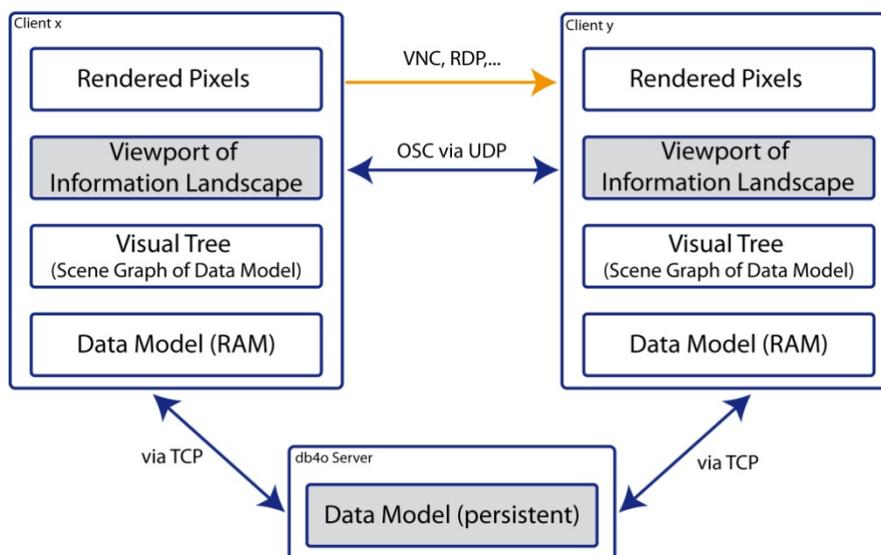
**Fig. 2.** Overview of ZOIL's distribution capabilities.
