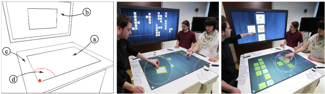
Figure 5. Workspace design: shared action space (a), reflection space (b), personal spaces (c) and transfer spaces (d).
