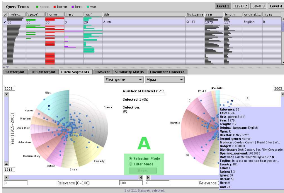
Figure 6. The CSV as a filter working in conjunction with VisMeBs other visualizations. Area 'A' shows the added UI elements. Selection of single documents: Selected and focused documents in the CSV are highlighted in the table. Tool-tips give details on demand.
