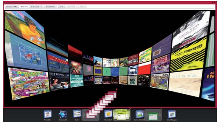
Zoomable user interface to manage multiple searches and baskets (tile scales are mapped to elapsed time).
