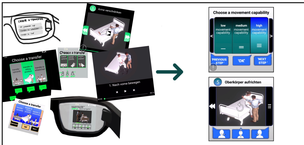
Figure 5.3.: Generative Design Process: Left side shows the ideation, sketching and refining of many early design possibilities. The screenshots on the right show the final design: the upper one shows a menu where a movement capability can be selected by interacting via voice commands and the bottom one shows an example of a video instruction that can be replayed or changed by interacting via head gestures.
