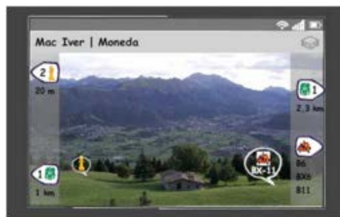
Figure 3.4: A Mock up of the interface of SidebARs is shown. Arrows with different types of off-screen objects are visualized on the sidebars. They are annotated with the closest distance and the amount of targets combined in one arrow (taken from [15]).
