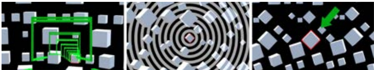
Figure 3.15: The techniques attention funnel (left), spherical wave based guidance (middle), and 2D arrow (right) are shown (taken from [6]).
