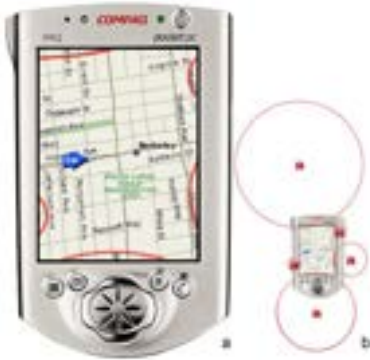
Figure 3.5: The figure visualizes five off-screen targets (a) and shows the circles that belong to the arcs (b) (taken from [1]).
