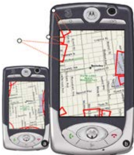
Figure 3.9: The Halo interface (a) and Wedge interface (b) are shown (taken from [4]).
