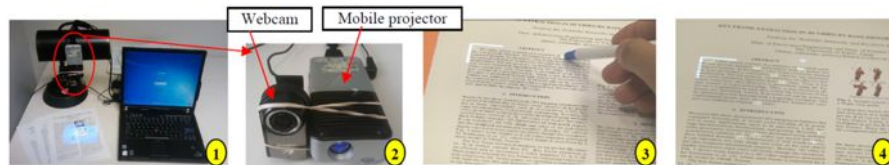
Figure 16: Fact prototype (1), close-up of the camera-projector unit (2), digital full-text search (3 a. 4) [41, p. 361].
