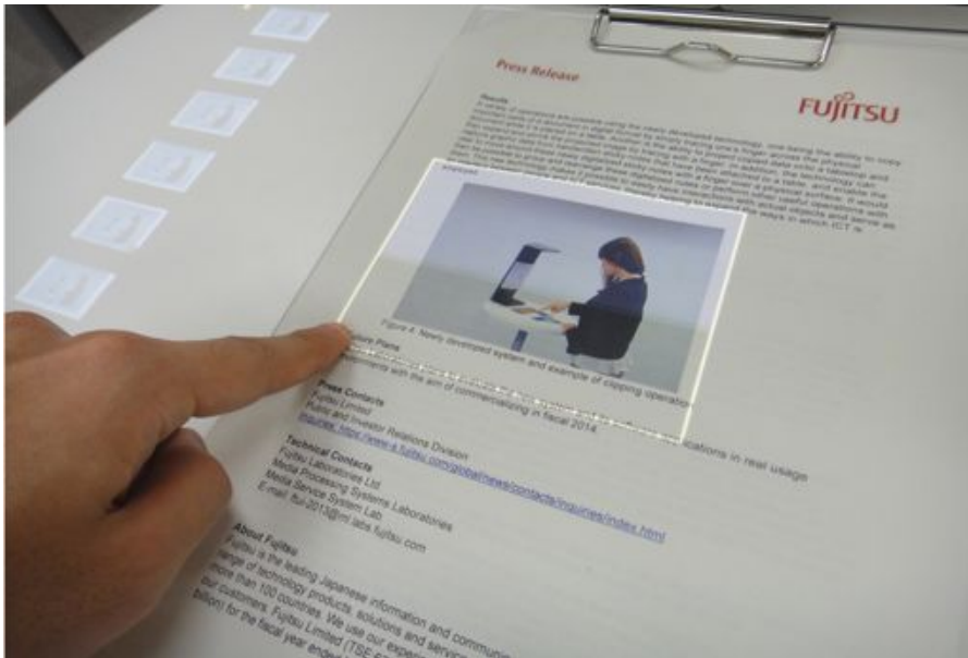
Figure 53: Fujitsu's system for interacting with real word objects like on touch-based computer systems.
