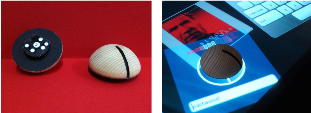
Figure 30: 2nd generation Search Tokens – Made out of wooden hemispheres. The Byte Tags are affixed on the bottom, which is blackened for a better detection of the tags by the tracking system.
