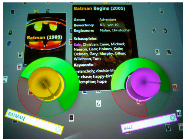
Figure 21: Two Search Tokens showing the concepts of sensitivity, weighted Booleans and color highlighting – The two movie objects in the center of the picture are larger than all other objects because they match one respectively two filter criteria defined by the yellow and the purple Search Token with the filter keywords "BATMAN" and "BALE". The keywords are highlighted in the detail information of the movie objects in the color of the corresponding Search Token.
