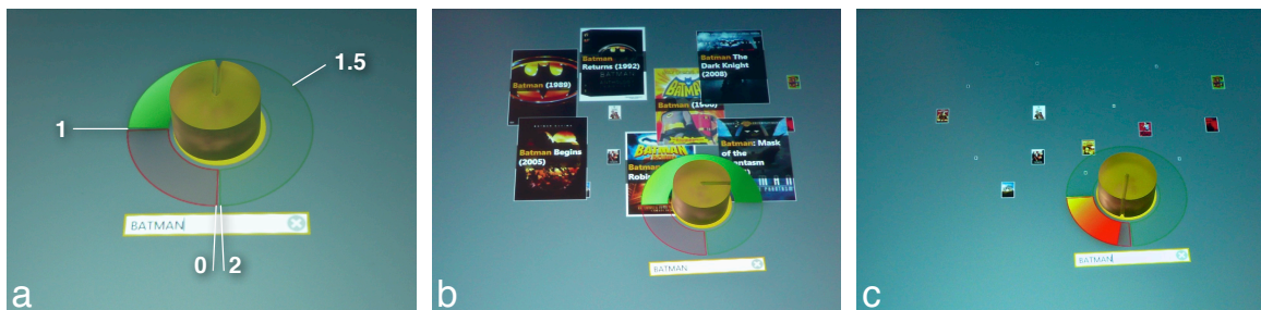
Figure 26: Weighting of a filter criterion – By turning the Search Token to the right and to the left, the weight of the filter is increased and decreased. a) The value ranges from 0 to 1 (red weight indicator part) and from 1 to 2 (green weight indicator part). The effect of altering the filter weight is that matching information objects will either increase their size (b) or decrease their size (c).
