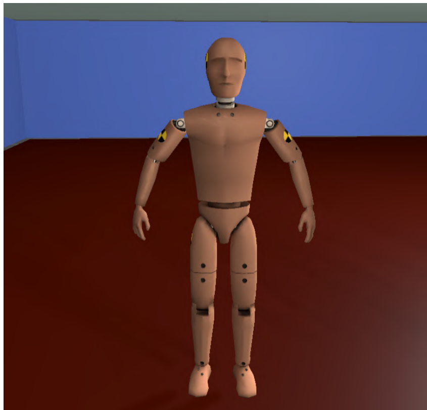
Figure 5.13.: Correctly configured inverse kinematics avatar for movement reproduction
