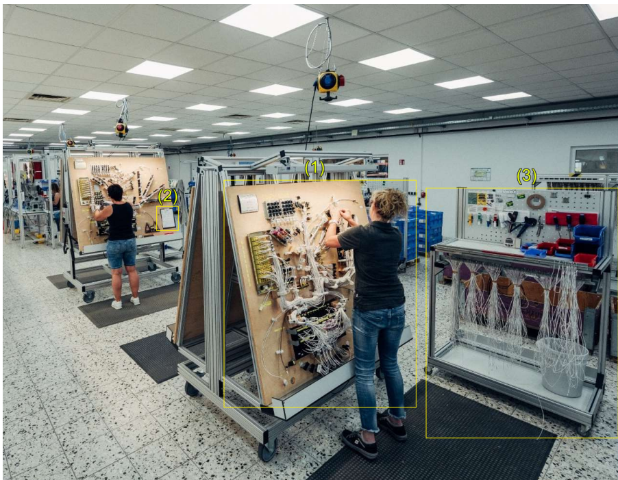
Figure 2.1.: Laying Board stations at Engeser with the laying board (1), the assembly instructions (2) and the cable cart (3) [1]
