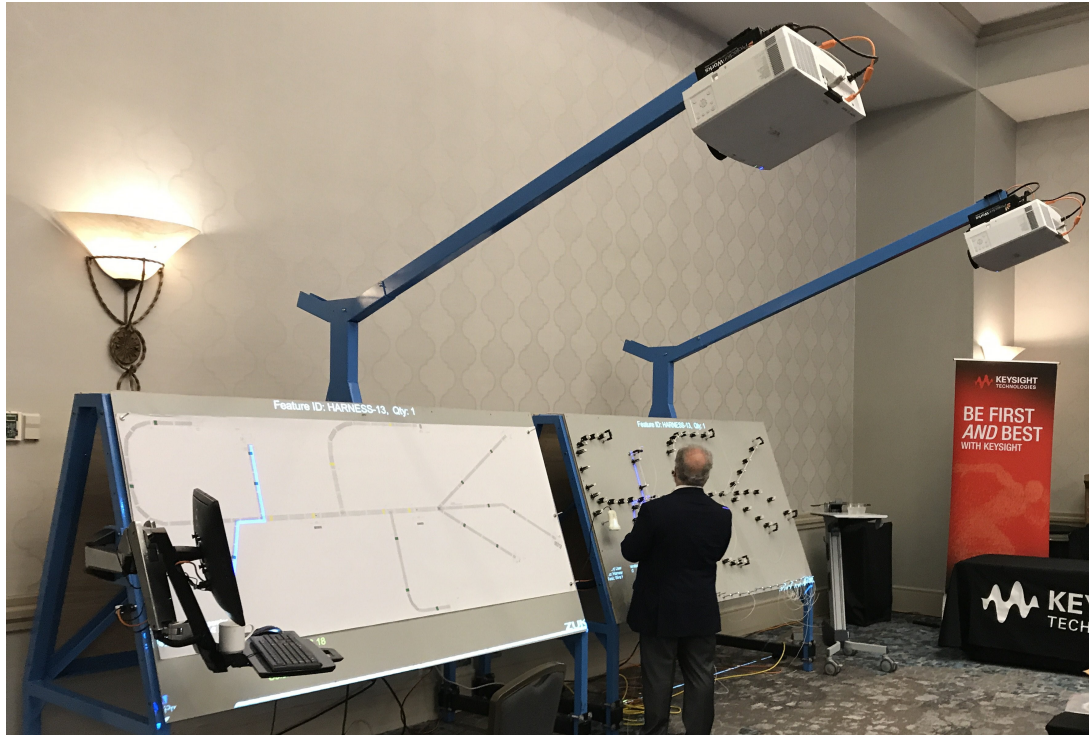
Figure 4.2.: Example of a Projector-Based System for Wire Harness Assembly [29]
