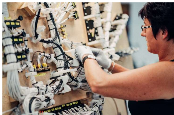
(b) Worker assembling a wire harness on a laying board [1]
