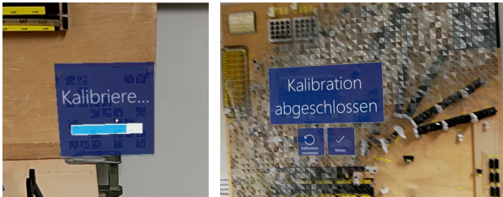
(a) The overlay that shows the current process of the calibration (b) After calibration has been completed, the user sees a pulsing overlay over the whole board that visualizes the calibration result
