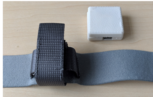
Figure 24 Final version: The sensor integrated into a chest strap with a case
