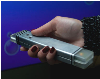
Figure 3: Well-known devices such as an omnipresent laser pointer enhanced with button module, LEDs and vibration motor provide flexible input from any distance. Users benefit from a more natural and convenient pointing experience.
