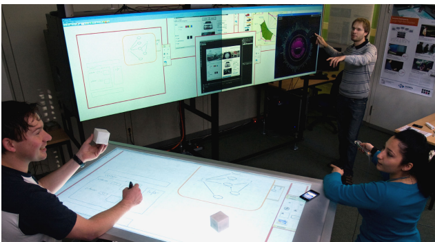
Fig. 13 The Media Room is a lab environment which provides a variety of input and output devices with different modalities and form factors. Squidy serves as the basic technology to integrate these different devices as well as to configure and evaluate them.
