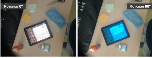
Figure 3. Both pictures show an image of the same scene taken by a camera with a polarization filter. The rotation of the polarization filter is 0^\circ in the first picture and 90^\circ in the second picture.
