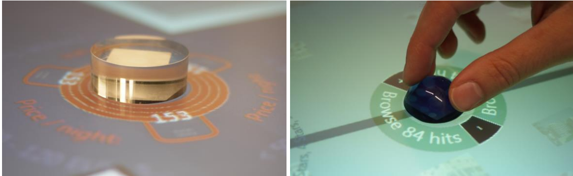
Figure 126 – A facet token (left) and a result token (right). Source: (Jetter, Gerken, Zöllner et al. 2011).
