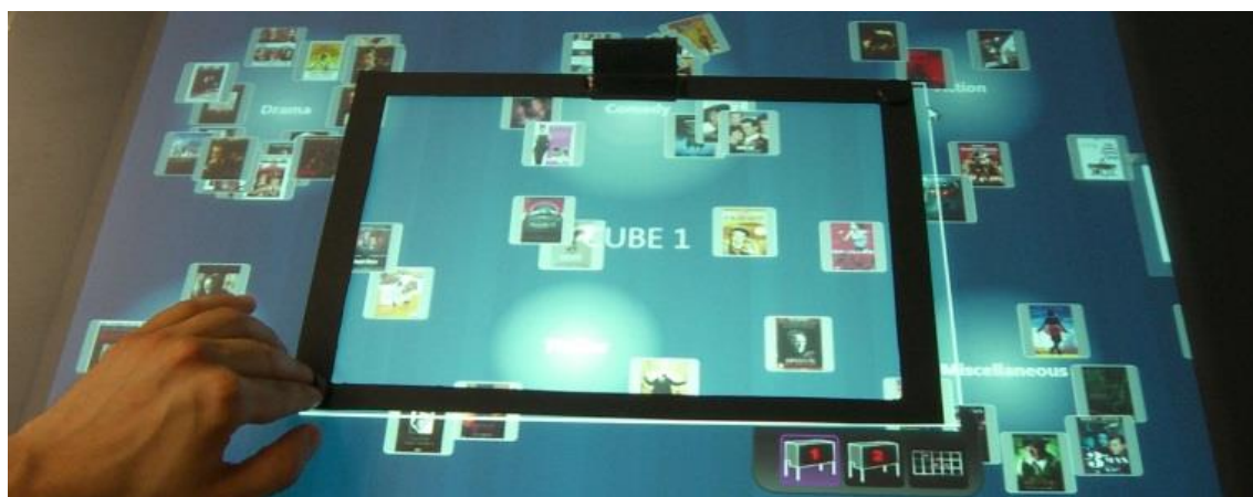
Figure 16 – The physical camera lens object on the tabletop can be used to establish coupling between the content that lies within the boundaries of the lens and the remote vertical displays.
