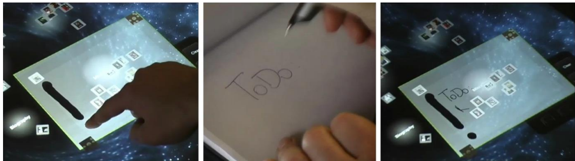
Figure 20 – Adding virtual Post-It notes using the ‘Post-It’ lens, touch input, and digital pen and paper.
