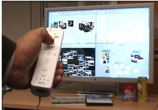
Figure 76 - Physical setup of EuroITV demonstrator with Wiimote controller and distant 30" high-resolution display 49 .
