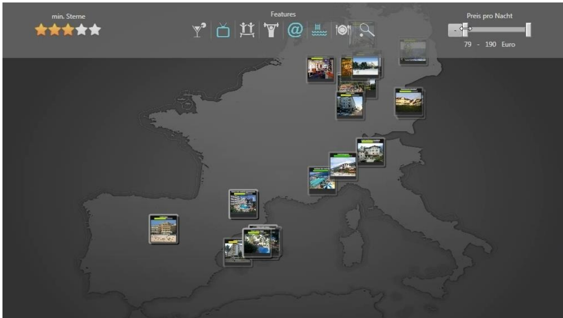
Figure 123 – The ZOIL-based HotelBrowser prototype uses dynamic queries at the top of the screen to filter the hotel objects in a map. Details of the hotels can be accessed using semantic zooming.
