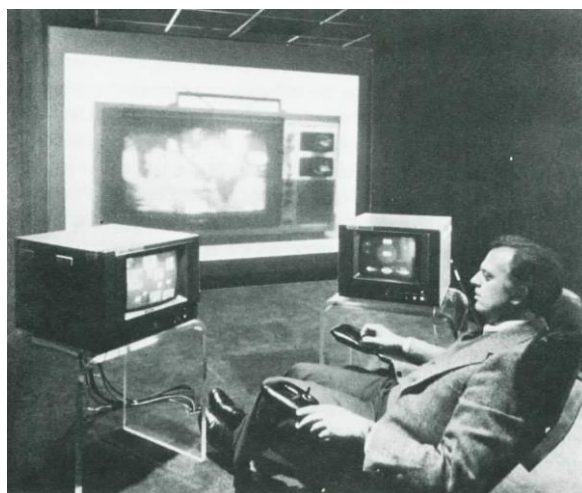
Figure 64 – The “Media Room” of the MIT running the ‘Spatial Data Management System’ on a large projector screen and two smaller touch-enabled monitors. Source: ( Bolt 1984 ).
