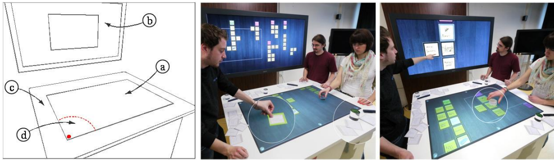
Figure 60 – The AffinityTable consists of a tabletop as shared action space (a) and a vertical 4K high-resolution display as shared reflection space (b). Source: (Geyer, Pfeil, Höchtl et al. 2011).
