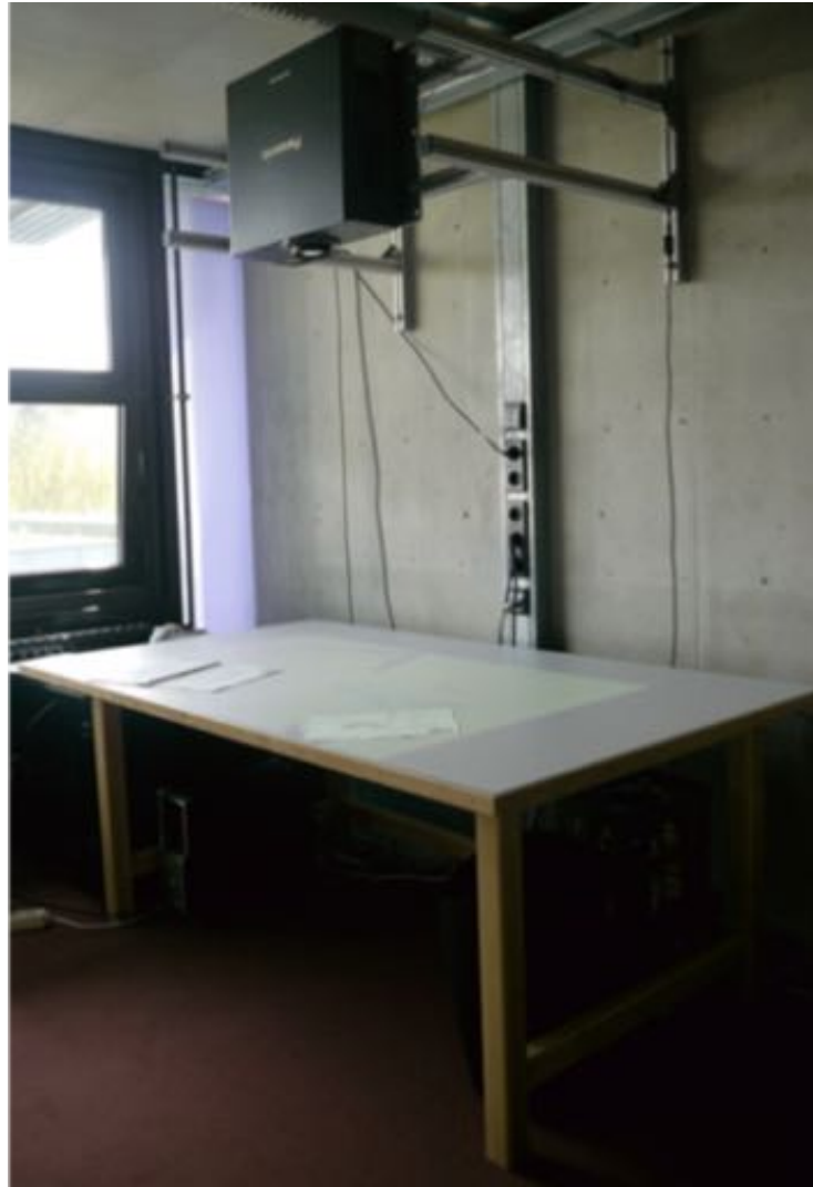
Figure 3.19.: Technical setup of Integrative Workplace consisting of a 100" interactive tabletop (pen & touch enabled), a camera to track documents put on the table surface and a projector to augmented the table and documents likewise. (adapted from (Gebhardt, 2013, p. 43))
