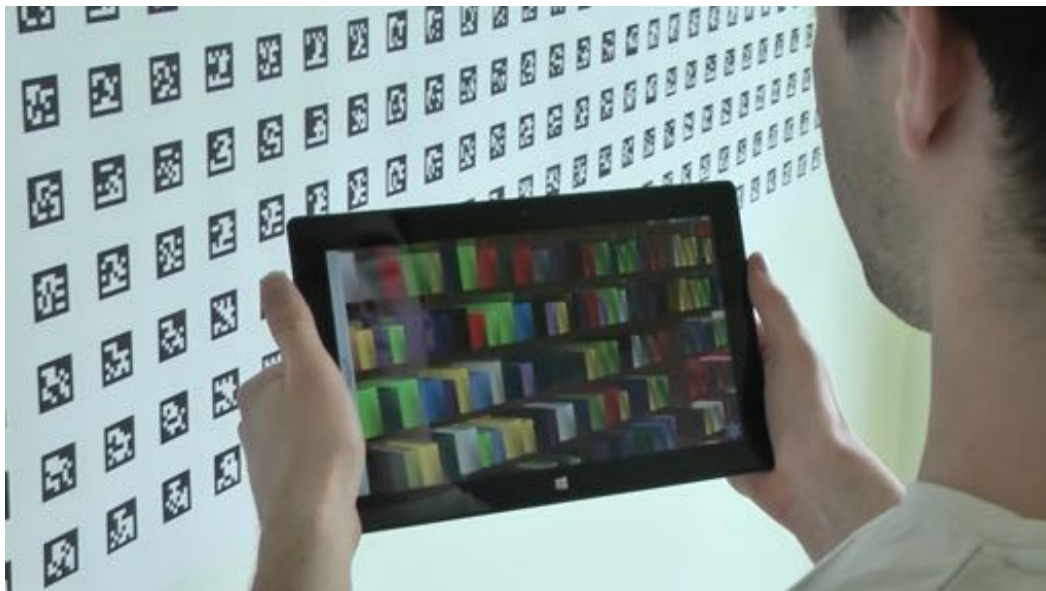
Figure 3.16.: The ShelfHole concept. Spatially-aware displays (peephole interaction) for reality-based exploration of library collections.
