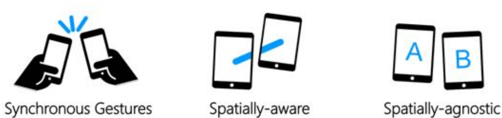
Figure 7.1.: Three identified cross-device gesture categories: Synchronous Gestures, Spatially-Aware Gestures, and Spatially-Agnostic Gestures.
