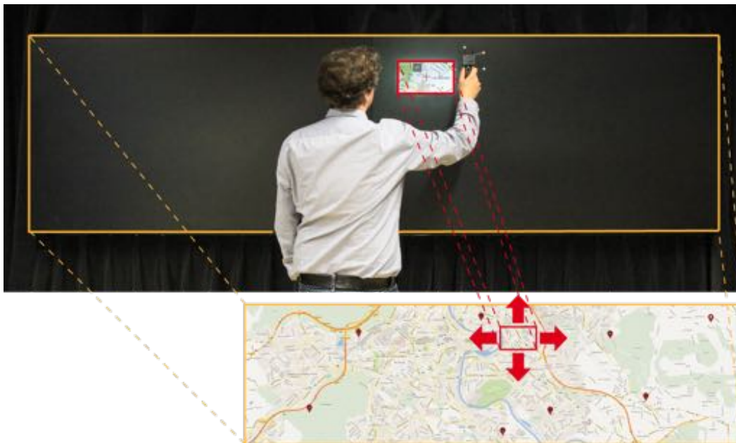
Figure 4.3.: Experimental setup simulating dynamic peephole interaction on a large vertical screen. This simulation allows to study the effect of peephole size on map navigation with high internal validity. It avoids confounding factors like weight and resolution of particular devices.
