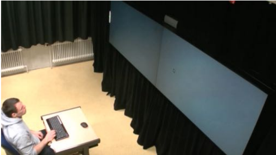
Figure 5.6.: A participant performing the recall task. He is seated at the mobile desk and provided with a keyboard. Participants used the arrow keys of the keyboard to move objects to recalled positions and place them with the enter key.
