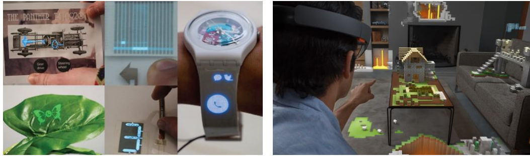
Figure 2.6.: Examples of future UbiComp systems, which promise to create cheap and disposable UbiComp devices or simulate entire UbiComp environments. Left is PrintScreen allowing fabrication of thin touch-displays (Olberding et al., 2014) and right is Microsoft HoloLens showing Minecraft Demo.
