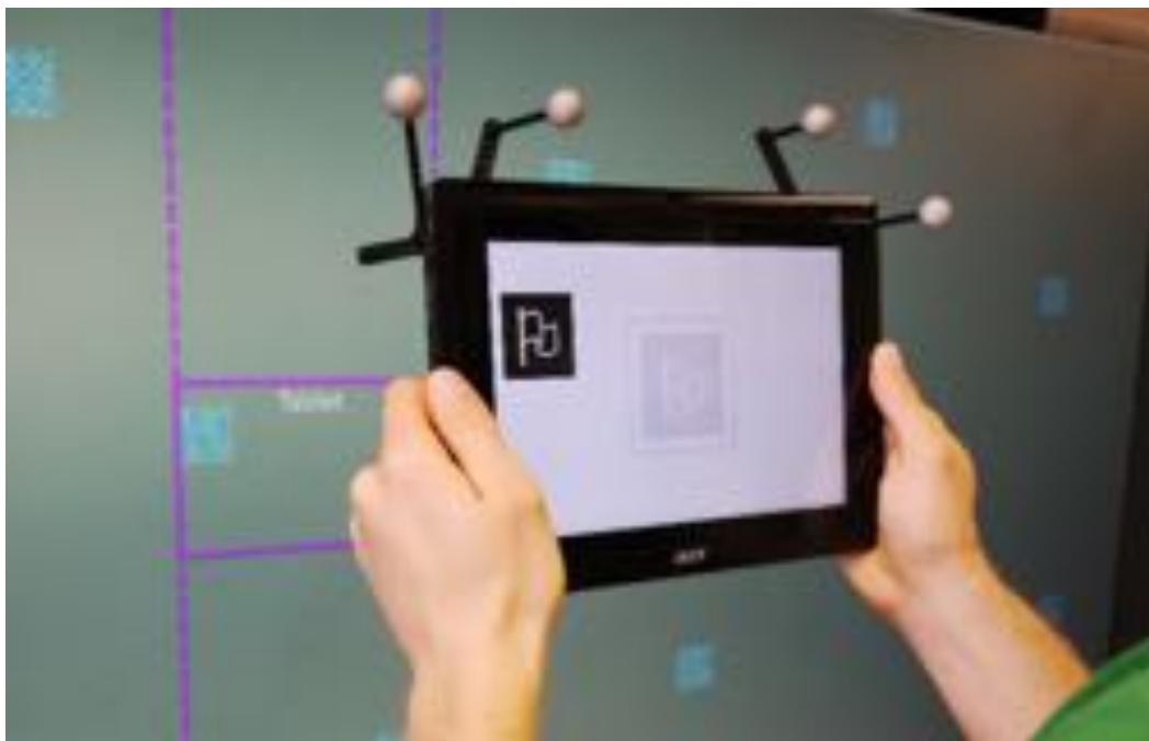
Figure 5.5.: A user navigating in the large canvas using the egocentric navigation. The purple rectangle on the overview display indicates the current position of the viewport on the large canvas.
