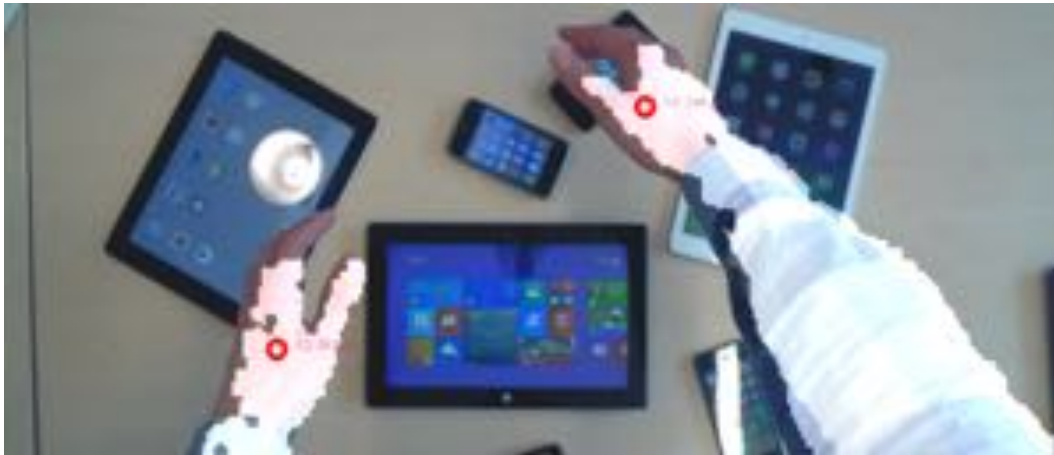
Figure 6.6.: Segmentation of hands and arms (white overlays) and estimated location and height of hands (red circles).
