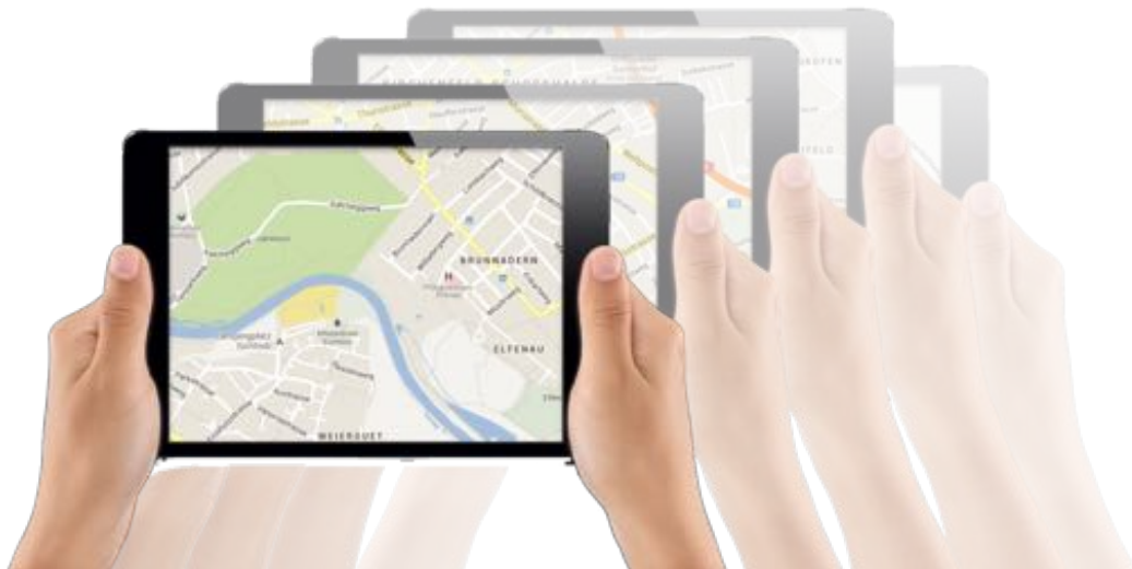
Figure 3.17.: Example of peephole interaction. Movements of a mobile display in physical space pans and zooms virtual content displayed on the mobile device's screen.
