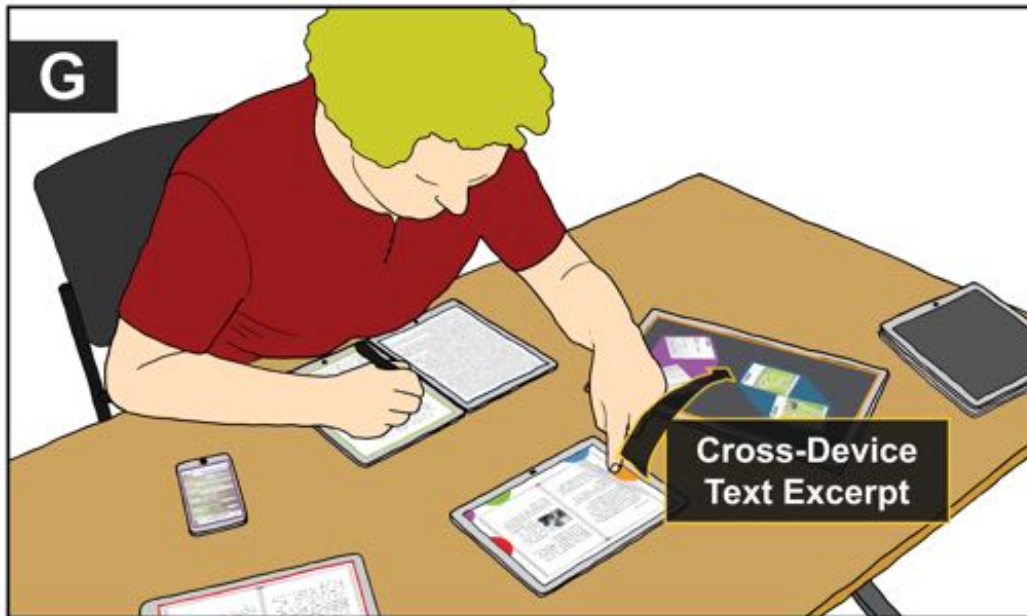
Figure 8.3.: Information is shared across devices using spatially-aware cross-device interactions such as edge bubbles.
