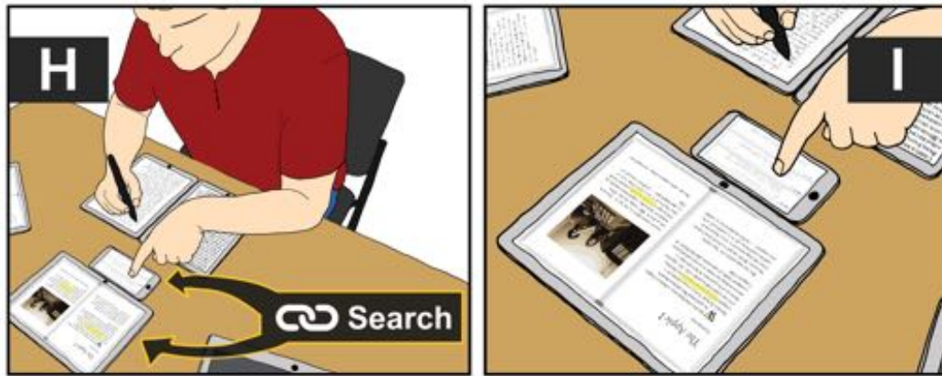
Figure 8.4.: Devices such as smartphones act as tools or instruments to manipulate views or substances displayed on spatially distant devices. In this case, a smartphone triggers keyword search in the next-by tablet and further list all search results. Tapping on a search result opens the corresponding page on the tablet.
