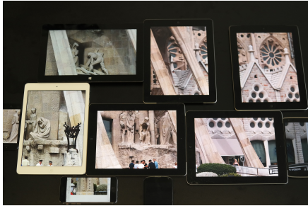
Figure 4: Example application. A high-resolution image is distributed across a large number of devices. Panning gestures are synchronized across all devices.
