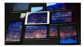
Figure 1.1: Many devices in complicated alignment form a connected display showing a dynamic high resolution image. Connected with Connichiwa. - Source: https://youtu.be/FEzxv-CMsAs?t=1m44s
