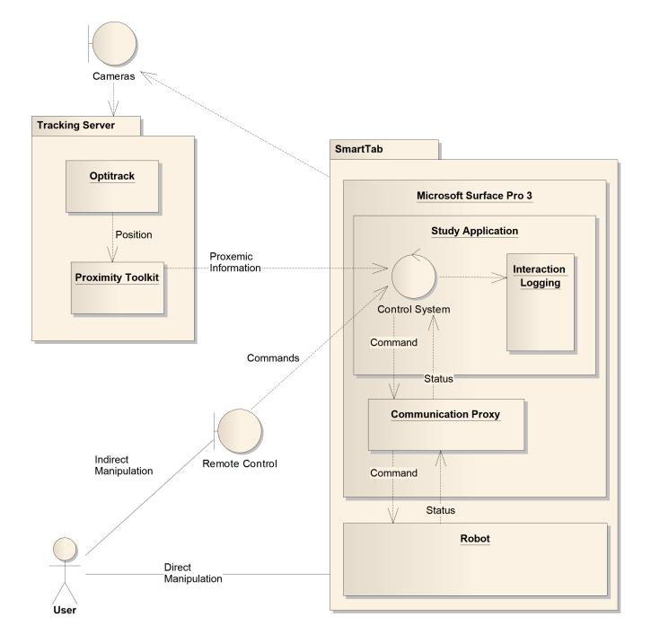
Figure 7.3: Overview of the study softwares components and the flow of information.
