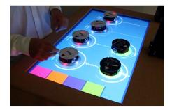
Figure 2.13: TangibleBots on top of a multitouch-table visualize a music mixer - Source: (Pedersen and Hornbæk 2011)
