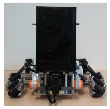
Figure 3.9: Front view showing the reinfoced lifting arm with the black anti-slip mat.
