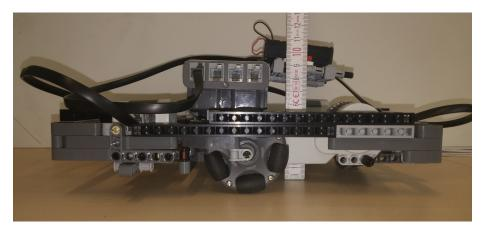
Figure 3.3: Side view of version 1b 14:20 illustrating the almost seesaw like design of the onmi wheel drive.
