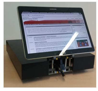
Figure 3.10: The SmartTab fully assembled with the black box and a Samsung Galaxy Tab S 10.5 mounted on the lifting arm.
