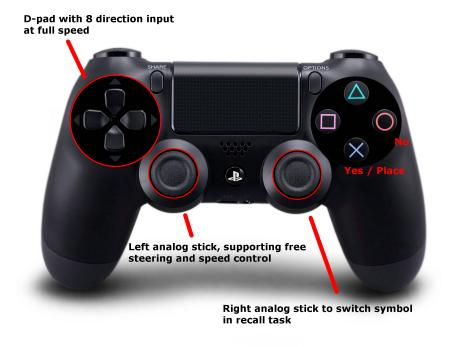
Figure 4.4: The Dualshock 4 controller with indications of the functions in the experiment.
