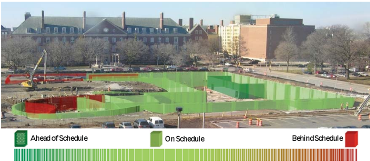
Figure 2.2: Prototype by Golparvar-Fard et al. (2009). MRE for the visual display of construction plans in a construction site (top) and visual highlighting of the current progress of the construction (bottom).
