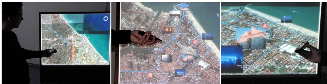
Figure 2.2: The interaction concept presented by Throw and tilt, using the smartphone orientation sensors [7]
