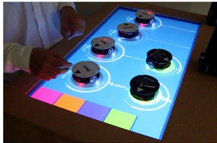
Figure 2.13: TangibleBots on top of a multitouch-table visualize a music mixer - Source: (Pedersen and Hornbæk 2011)
