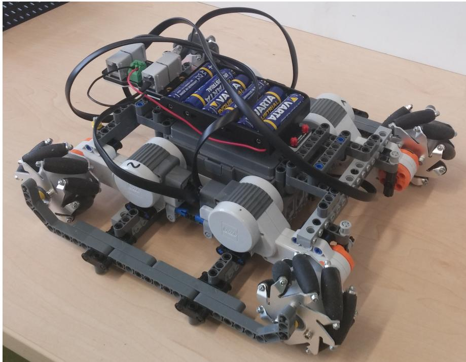
Figure 3.1: Bird view of version 1a with the mecanum wheels.
