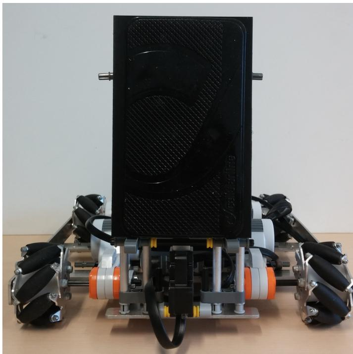
Figure 3.9: Front view showing the reinforced lifting arm with the black anti-slip mat.
