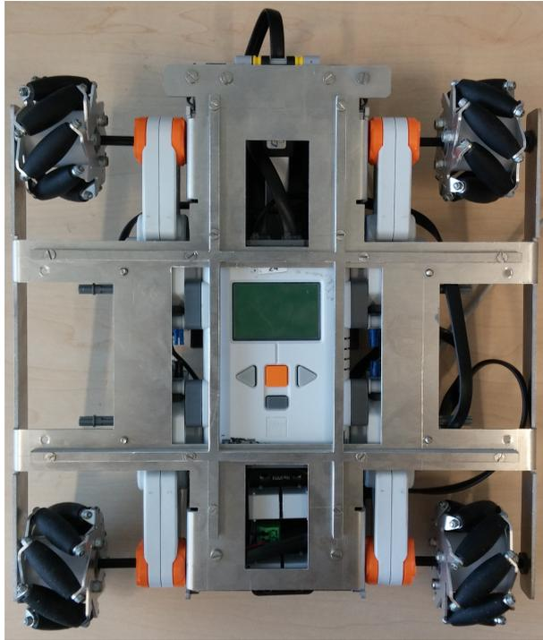
Figure 3.8: Bottom view showing the skeletal reinforcement structure.
