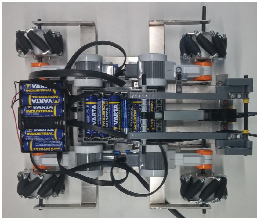
Figure 3.6: Top view of the fully assembled prototype 2. The long axles allow to chose the best position for the mecanum wheels.
