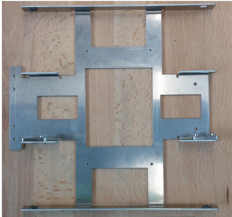
Figure 3.7: Improved frame. Showing the connected sides and rounded edges. Also two axle mountings are attached.
