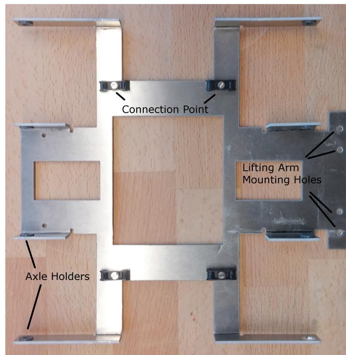
Figure 3.5: The bare aluminium frame. The four screwed on black Lego pieces connect the frame with the motors and the NXT.
