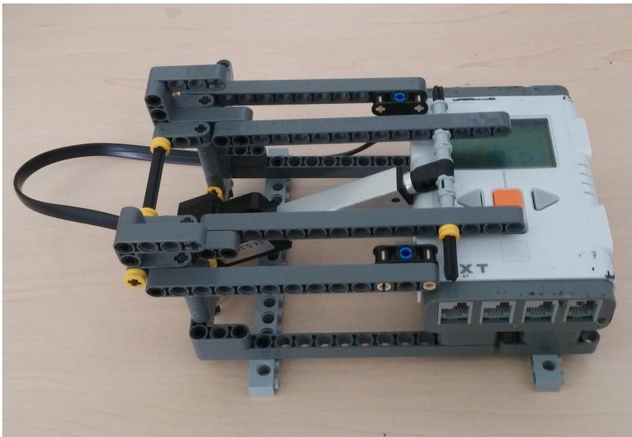
Figure 3.4: Display of version 1c without a tablet lying on it. The silver linear actuator is clearly visible in the middle of the lever.
