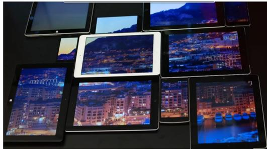
Figure 1.1: Many devices in complicated alignment form a connected display showing a dynamic high resolution image. Connected with Connichiwa. - Source: <https://youtu.be/FEzxxv-CMsAs?t=1m44s>
