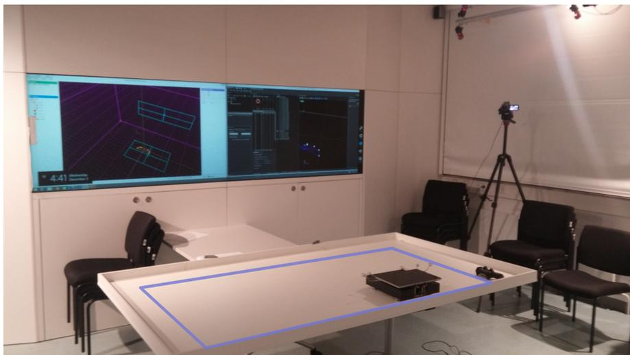
Figure 4.1: The experimental setting in the lab with the SmartTab sitting on the desk with the border. The blue outline indicates the approximate size of the virtual display.
