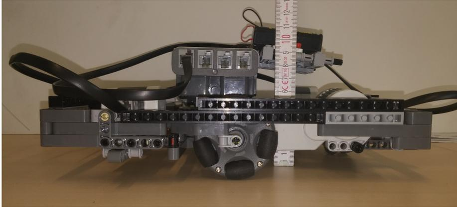
Figure 3.3: Side view of version 1b 14:20 illustrating the almost seesaw like design of the omni wheel drive.
