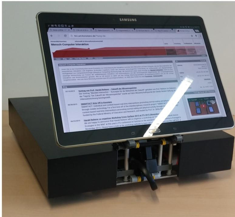
Figure 3.10: The SmartTab fully assembled with the black box and a Samsung Galaxy Tab S 10.5 mounted on the lifting arm.
