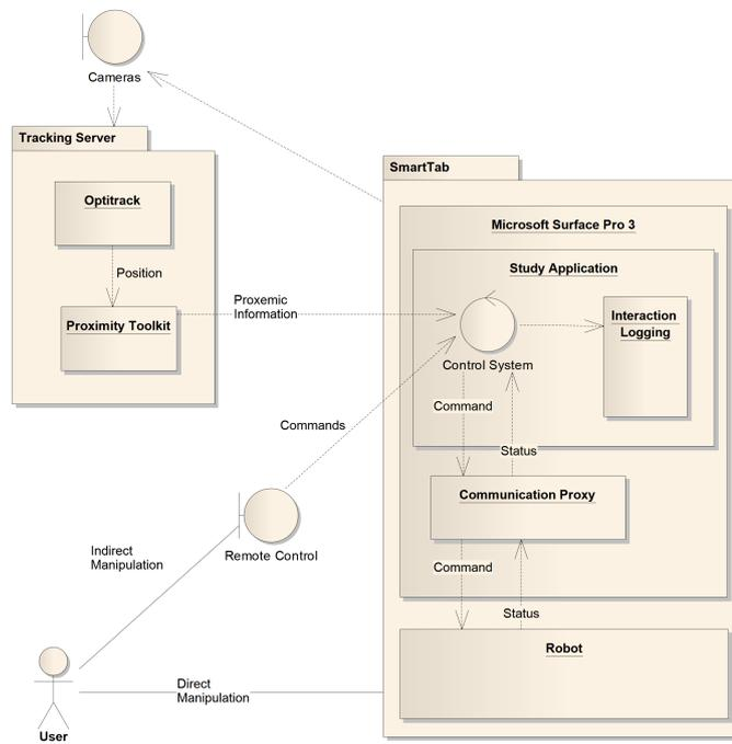
Figure 4.6: Overview of the study software architecture highlighting the main features. (Bigger picture in appendix 7.3)
