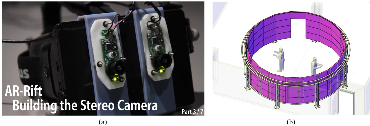
Figure 3.6: Hardware for immersive environments. (a) The AR-Rift project uses a VR HMD with two front-mounted cameras for stereoscopic vision [78]. (b) Concept drawing of a CAVE2 system, where users are fully surrounded by monitors with a thin bezel [30].
