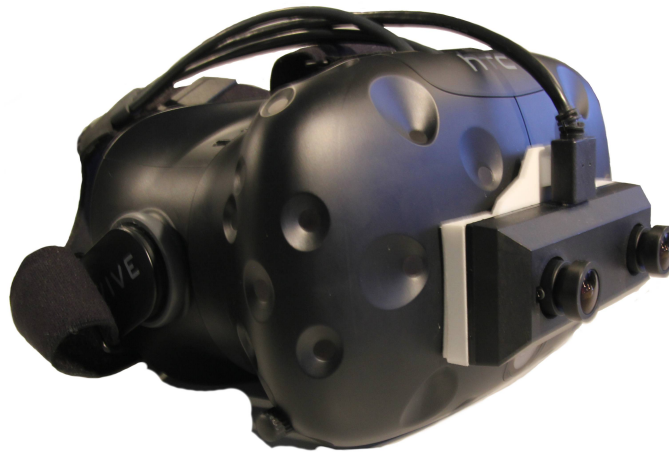
Figure 4.8: HTC Vive HMD with front-mounted OvrVision Pro cameras.
