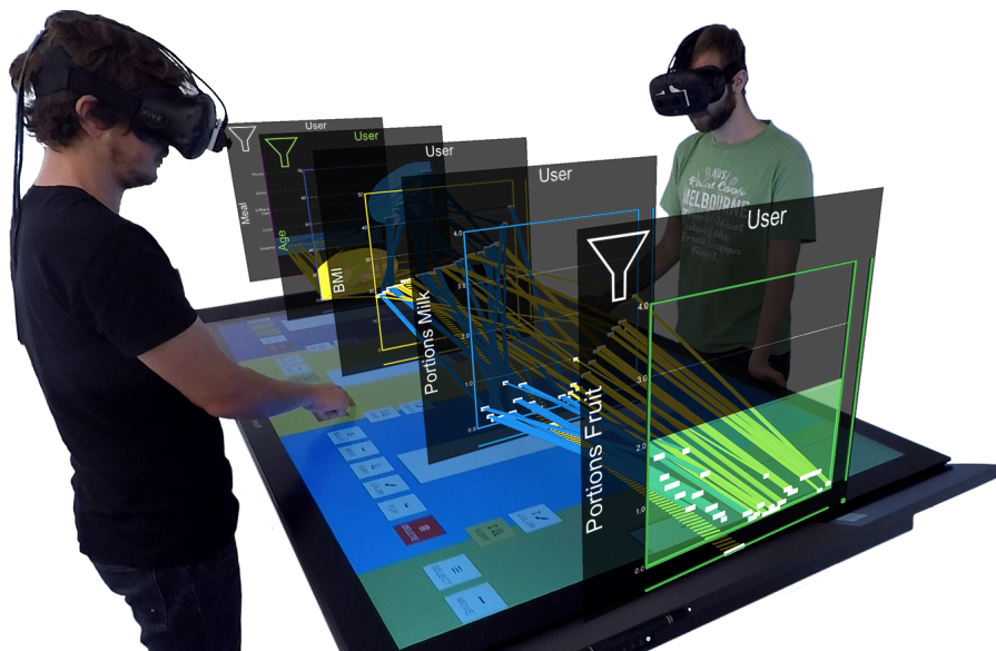
Figure 4.1: The ART prototype uses a VR HMD with front-mounted stereoscopic cameras to visualise 3D parallel coordinates above a touch-enabled tabletop.
