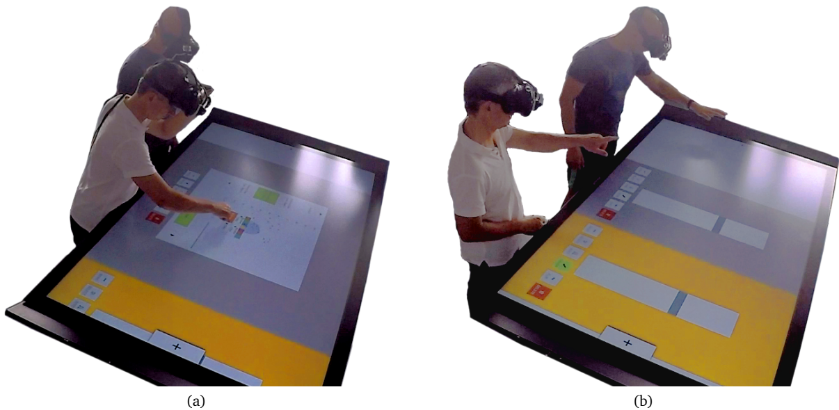
Figure 5.4: Due to the limited camera quality, some users had to take off the HMD when interacting with the table. (a) User on the left takes off HMD to interact with table. (b) User on the left wears HMD again to look at the AR visualisation.
