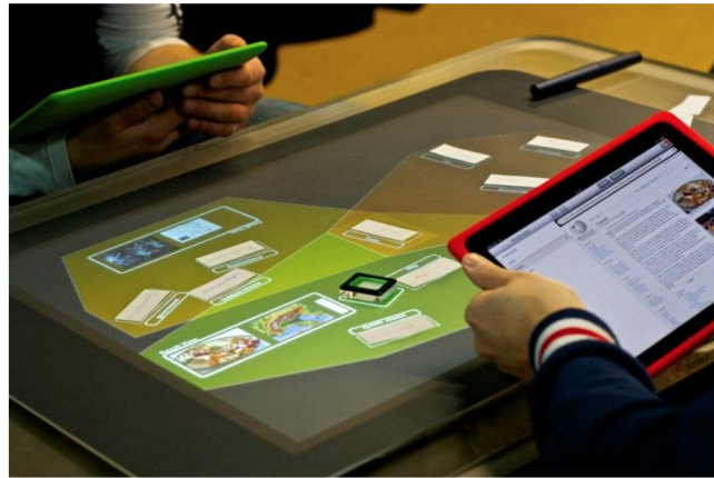
Figure 5: TwisterSearch during usage, showing the personal tablet of a user and the shared tabletop. A tablet-shaped token on the tabletop indicates that the cluster it is placed on is owned by the tablet of the same colour. Source: [73]
