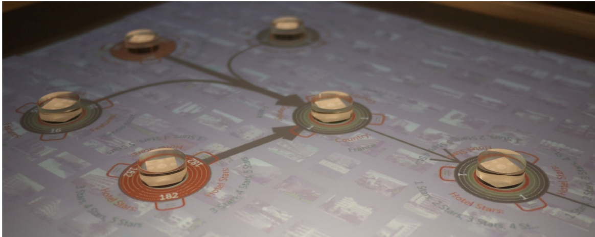
Figure 6: FacetStreams with multiple tokens. Directed streams connect the tokens. When a stream goes through a token, it is filtered by the tokens attached metadata and value range. Source: [37]
