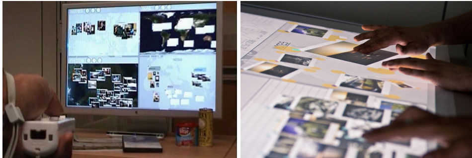
Figure 18: The left picture shows the iTV prototype in use with a Wiimote. To the right, the same interface is displayed on a multi-touch table.
