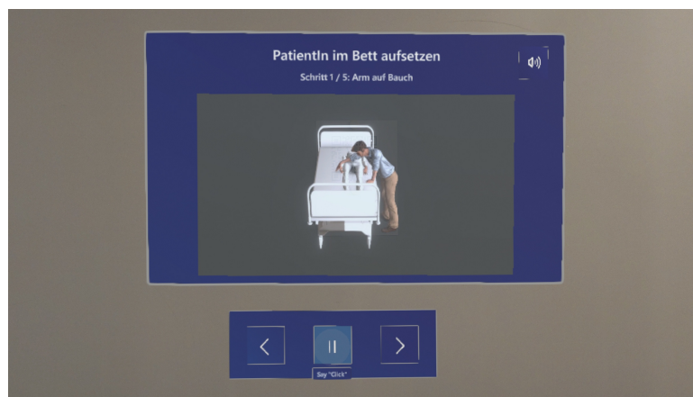
Figure 4.13: User interface of the interaction technique eye gaze and voice. The gaze is currently pointing at the pause button and the user receives visual feedback. The selection can be confirmed by saying the voice command.
