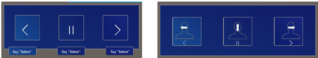
Figure 4.12: Control panel of eye gaze and voice on the left and head gestures on the right.
