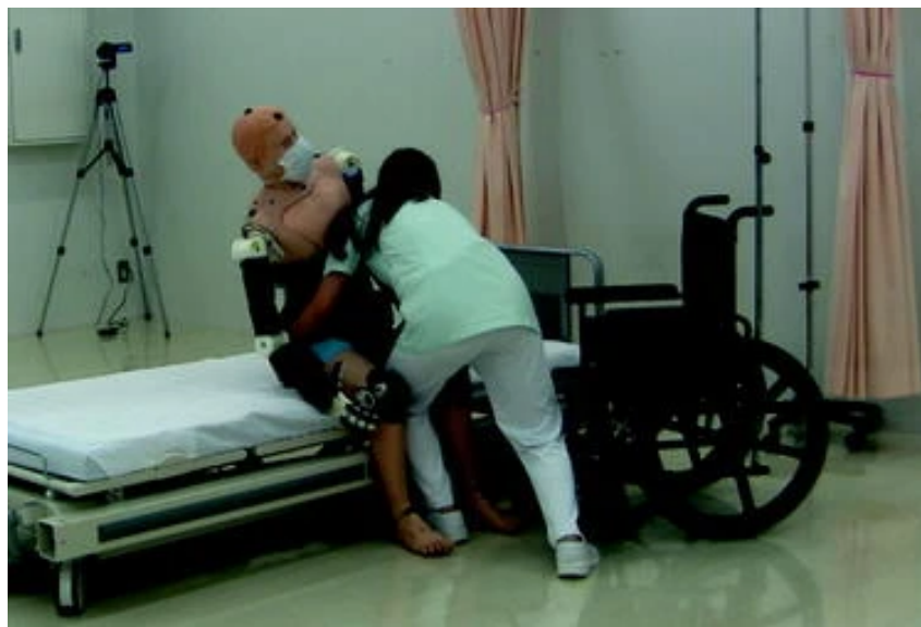
Figure 2.2.: The robot that was used by Nakamura et al. as a substitute for a human.[10]
