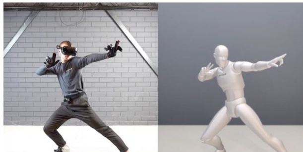
Figure 3.6.: Vive tracker setup
