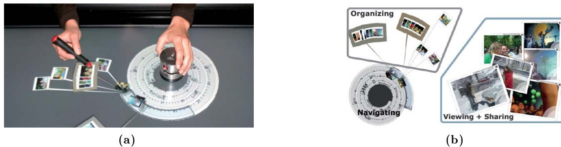
Figure 3.8: PhotoHelix [28]: (a) Spiral-shaped time-based visualization with its physical control and the pen as input device. (b) Organizing, navigating and sharing of pictures.
