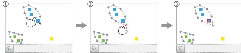
Figure 4.18: (1) Touching and dragging the handle. (2) Releasing the handle. (3) Resizing the object in the bin.
