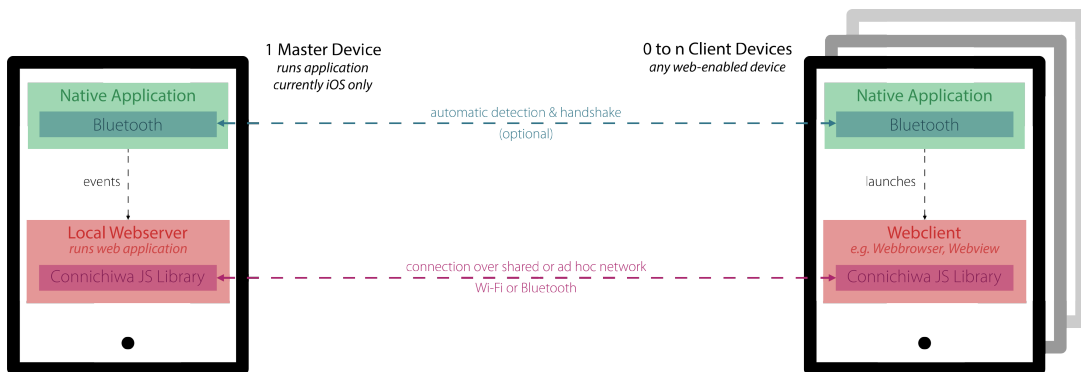
Figure 11: In addition to WebSocket communication (see Figure 10), client devices can run a native application and enable the full feature set of Connichiwa, such as ad hoc Bluetooth detection.
