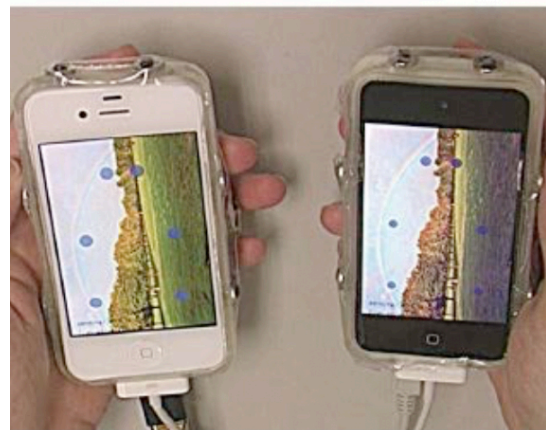
Figure 3: MagMobile (Huang et al. 2012) uses a custom magnetic sleeve for device detection. Source: (Huang et al. 2012) (parts of the image were cropped).
