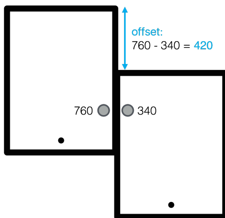
Figure 13: Offset calculation based on a synchronised swipe on two devices. The grey dots mark the y-locations of the two swipes with their local coordinates.
