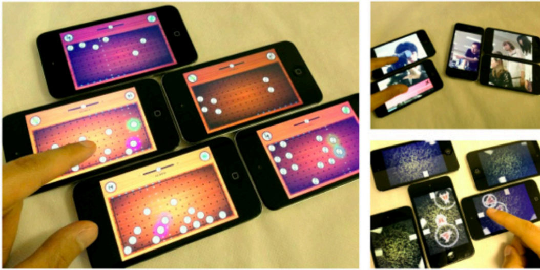
Figure 9: Example applications implemented using Pinch (Ohta and Tanaka 2012). After pinching, stitched user interfaces across multiple devices are enabled. Source: (Ohta and Tanaka 2012).
