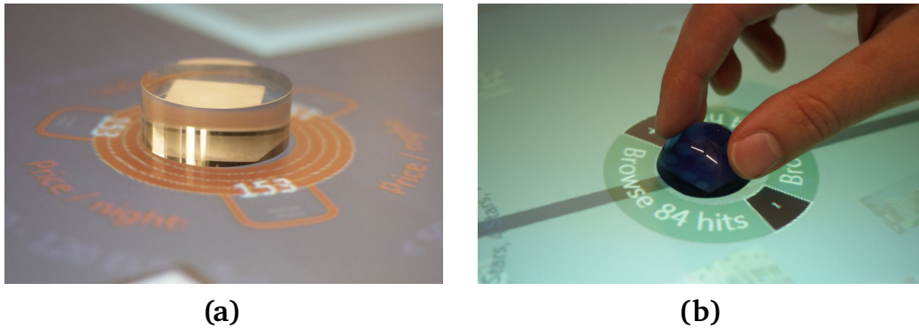
Figure 3.3: Facet-Streams binds digital filters to different physical tokens [68]. (a) Each token represents a filter that can be configured through touch. (b) A differently shaped token allows users to view the results.
