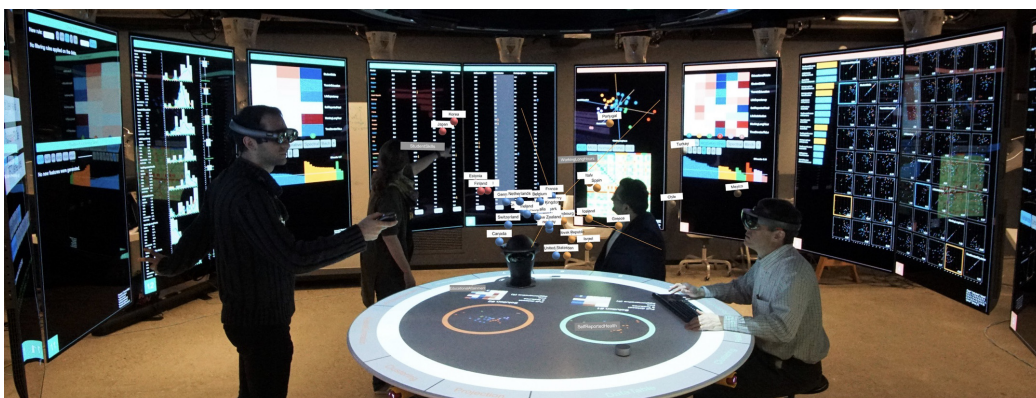
Figure 4.8: Immersive Insights leverages a hybrid reality environment to display several data views, combining large displays, projectors, and immersive AR devices [23].
