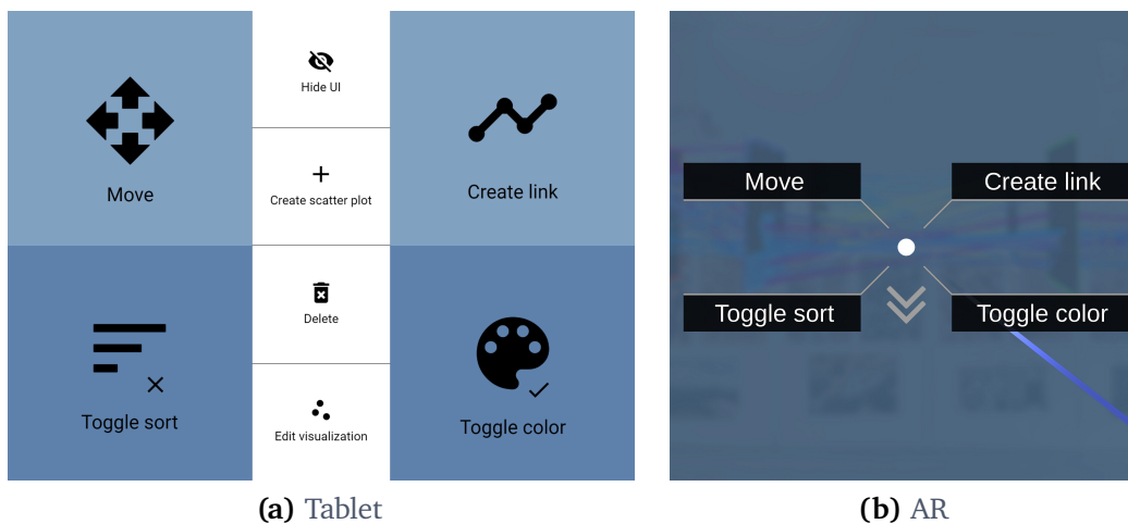
Figure 5.4: (a) Tablet menu with four interaction zones in each corner for eyes-free interaction. Further actions are available in the middle, which require the user to look at the tablet. (b) The menu entry of each corner is displayed in an AR head-up display (HUD), so that the user can interact with the tablet without looking at it.
