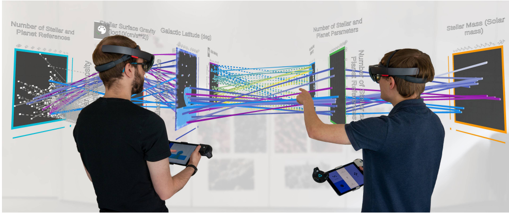
Figure 1.1: MIDAiR displays a 3D visualisation in an immersive AR environment. A spatially-aware tablet and an AR HMD offer multimodal input for interacting with the visualisation.
