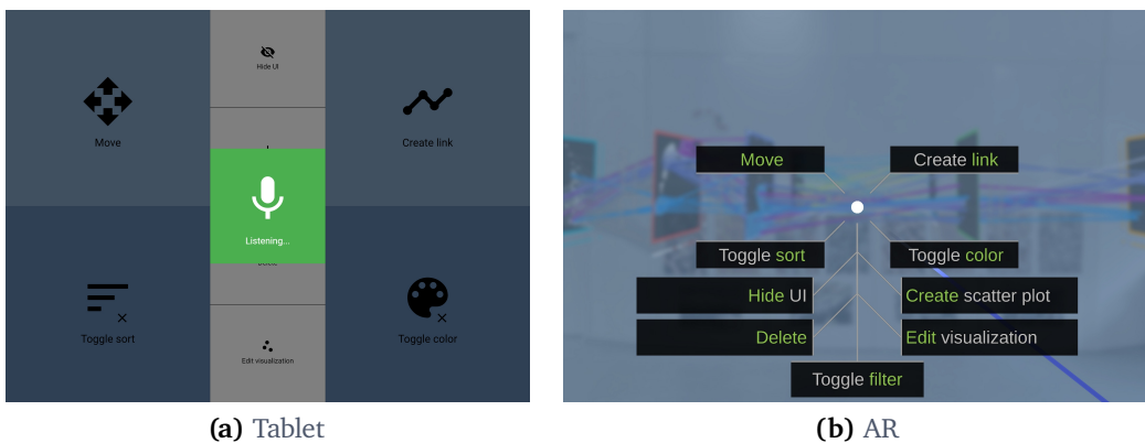
Figure 5.14: MIDAiR adjusts the interface when voice commands are active. (a) On the tablet, an indicator shows that the application is now listening, fading out the other interaction elements. (b) The AR HUD displays all available actions, highlighting the voice activation keywords in green.
