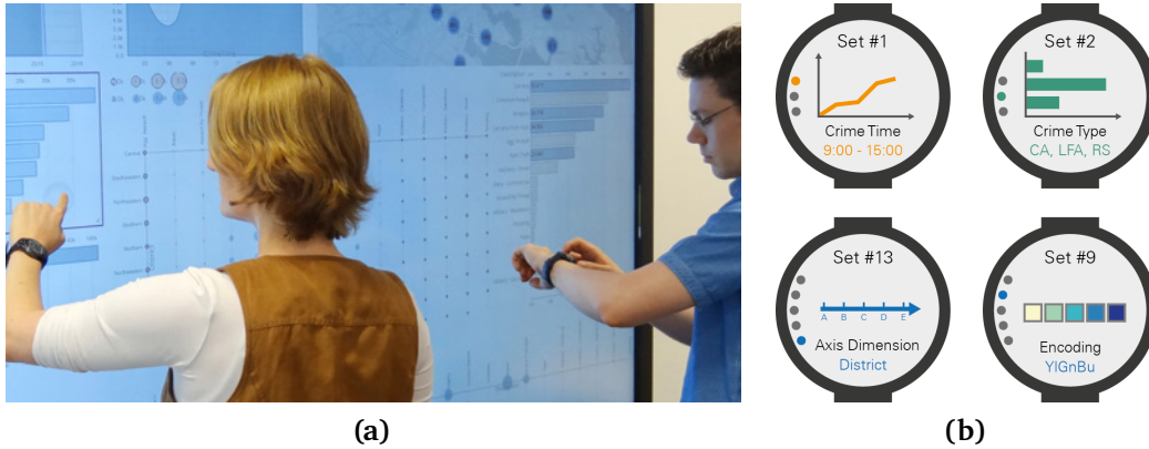
Figure 4.4: When David Meets Goliath combines smartwatches with a large display [56]. (a) Users can select visualisation through touch on the display and interact with the visualisation on the smartwatch. (b) Content can be stored on the smartwatch, such as filters, dimensions, or encodings.
