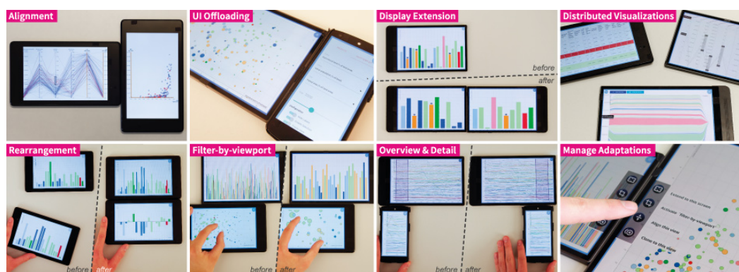
Figure 4.2: VisTiles uses mobile devices to display and control visualisations. Devices can be combined in different ways, depending on their orientation [77].
