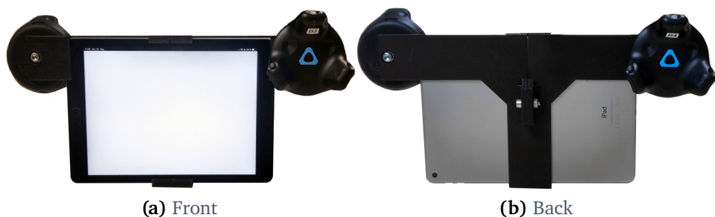
Figure 6.2: For interaction, MIDAiR uses an iPad Pro tablet. To make this tablet spatially aware, a custom 3D printed frame was attached to the tablet and HTC Vive trackers were mounted to the frame.
