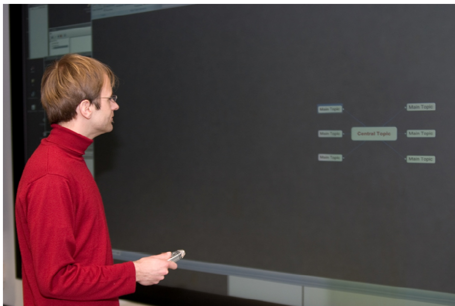
Figure 16. Using the motion-sensing laserpointer (wireless version) for gesture interaction and direct pointing with an electronic mind mapping application on the POWERWALL large high-resolution display
