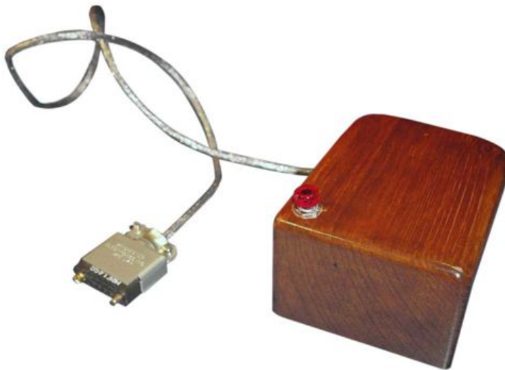
Figure 1.1: The first prototype of a computer mouse invented and developed by the Californian scientist Douglas Engelbart.
