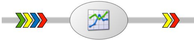
Figure 4.24: The pipe as it is implemented in Squidy. Each pipe has two data filters and a dataflow visualization on top.
