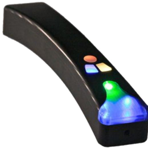
Figure 5.2: The laser pointer device consists of a IR laser diode, a button module, a vibrator, and led diodes.
