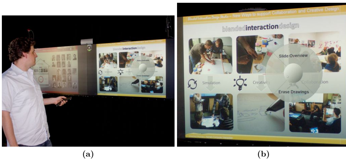
Figure 5.9: Impressions of the Powerpointer interaction technique: (a) an end-user employing the Powerpointer interaction technique, and (b) the pie menu reveals further actions available by the Powerpointer interaction technique.
