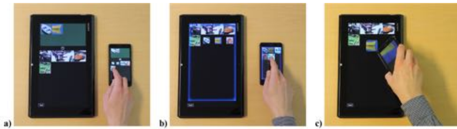
Figure 3.6: Multi-device object transfer. (a) Tray: a tray shared by all other devices. (b) Transfer mode: pair devices up to enable transfer of objects between them. (c) Device Touch: objects from one device could be moved into another by tapping of the origin phone onto the destination device. Source: (Jokela et al., 2015).
