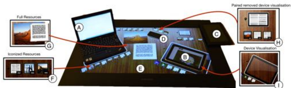
Figure 3.8: An example setup of the ActivitySpace. It contains a tabletop display (E), a laptop (A), a phone (D) and two tablets (B, C). All devices and documents associated with them are visible in the configuration space (H, I and F,G respectively). Source: (Houben et al., 2014).
