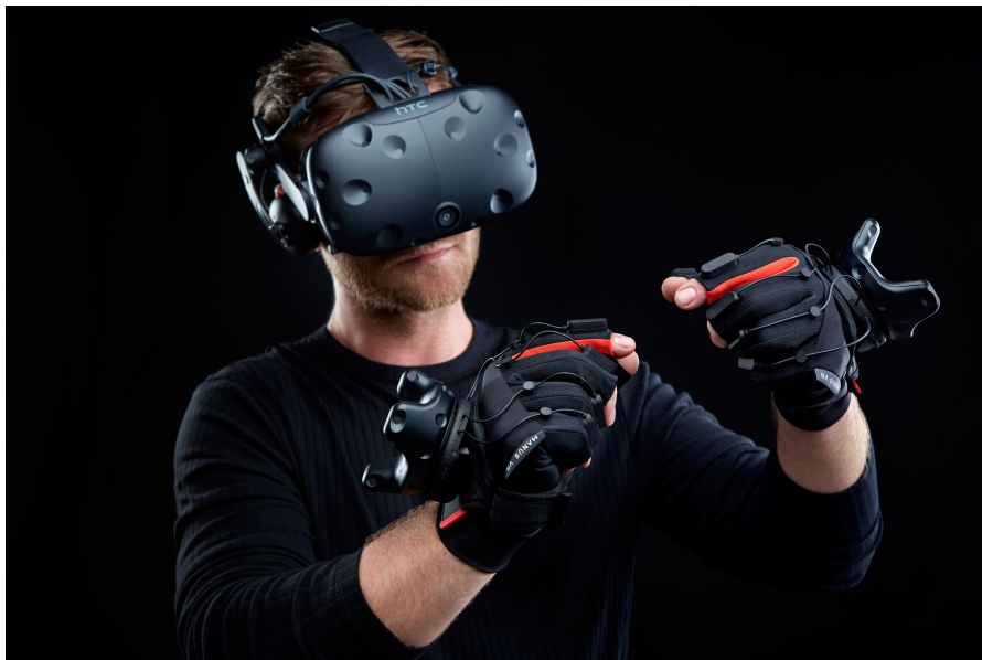
Figure 18: The ManusVR Prime Haptic gloves offer hand tracking and per-finger haptic feedback primarily for VR applications (ManusVR, < https://manus-vr.com/ >).
