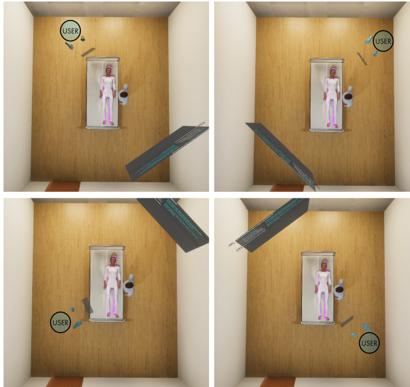
Figure 28: In mode 1, the information board switches between four different room positions, depending on the current user position. The information board always tries to be in the opposite room corner, respective to the user. There are buffer zones, so that erratic and confusing behaviour is mitigated. Additionally, the information board always directly faces the user through rotation. Those measures should ensure constant easy visibility.
