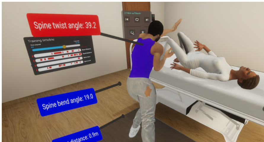
Figure 38: CaregiVR, a VR application focused on providing feedback on user's posture during a patient transfer.[37]
