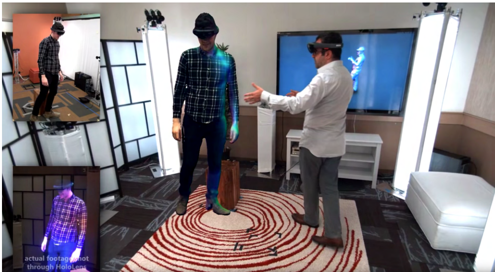
Figure 3.2.: The Holoportation system captures a user with multiple cameras and reconstructs the user in 3D. Wearing an AR HMD, the user at the remote site can see the 3D model of the user in real-time. Taken from [27].
