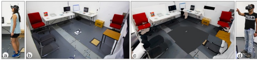
Figure 3.7.: The CoVAR [26] system setup. (a) shows the AR user and (b) her physical environment. (c) shows the reconstructed environment for the VR user and (d) the VR user. Taken from [25]
