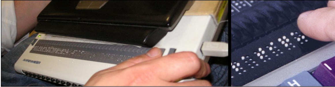
Figure 9: Left: A Braille display connected to a laptop. Right: Pin arrays (adapted from [BrailleNet 1998])
