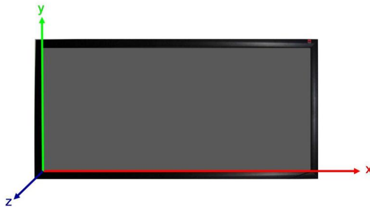
Figure 35: The “room coordinate system” of the optical tracking system installed at the Powerwall
