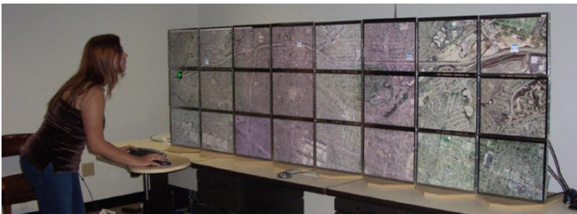
Figure 5: LHRD build with 24 tiled 17'' monitors, with a resolution of 96 DPI (taken from [Shupp et al. 2006])
