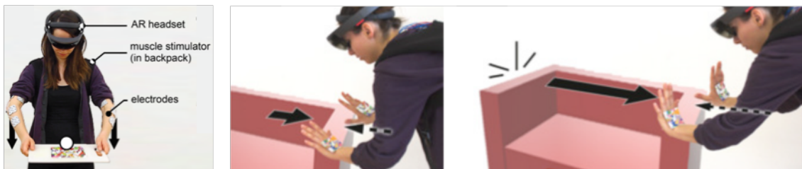
Figure 6.4: Lopes et al. [39] suggest electric muscle stimulation for haptic feedback in AR. Taken from [39].
