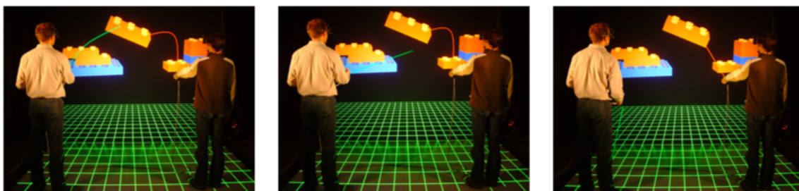
Figure 3.9: The Bent Pick Ray technique by Riege et al. [27] is based on ray-casting. To compensate for conflicting movements, it bends the rays of the users ( left ). As soon as one user releases the object, his ray get immediately unbent ( middle ). The ray of the other user gets unbent with further movement ( right ). Taken from [27].
