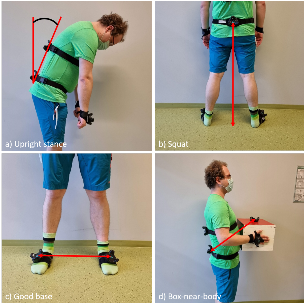
Figure 4.12.: Calculation of the risk metrics. a) upright stance – angle between the upright vector and the vector from the L5 tracker to the T8 tracker, b) squat – Euclidean distance between L5 tracker and floor, c) support base – Euclidean distance between the feet tracker, d) box-near-body – distance between L5 tracker and box tracker.
