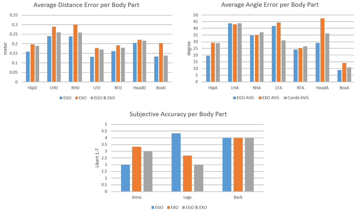
Figure 5.3.: Average error per body part. Left: distance error, right: angle error. Suffix D: distance, suffix A: angle. LH - left hand, RH - right hand, LF - left foot, RF - right foot. Bottom: subjective accuracy per body part, rated on a Likert scale 1 (best) - 7 (worst).
