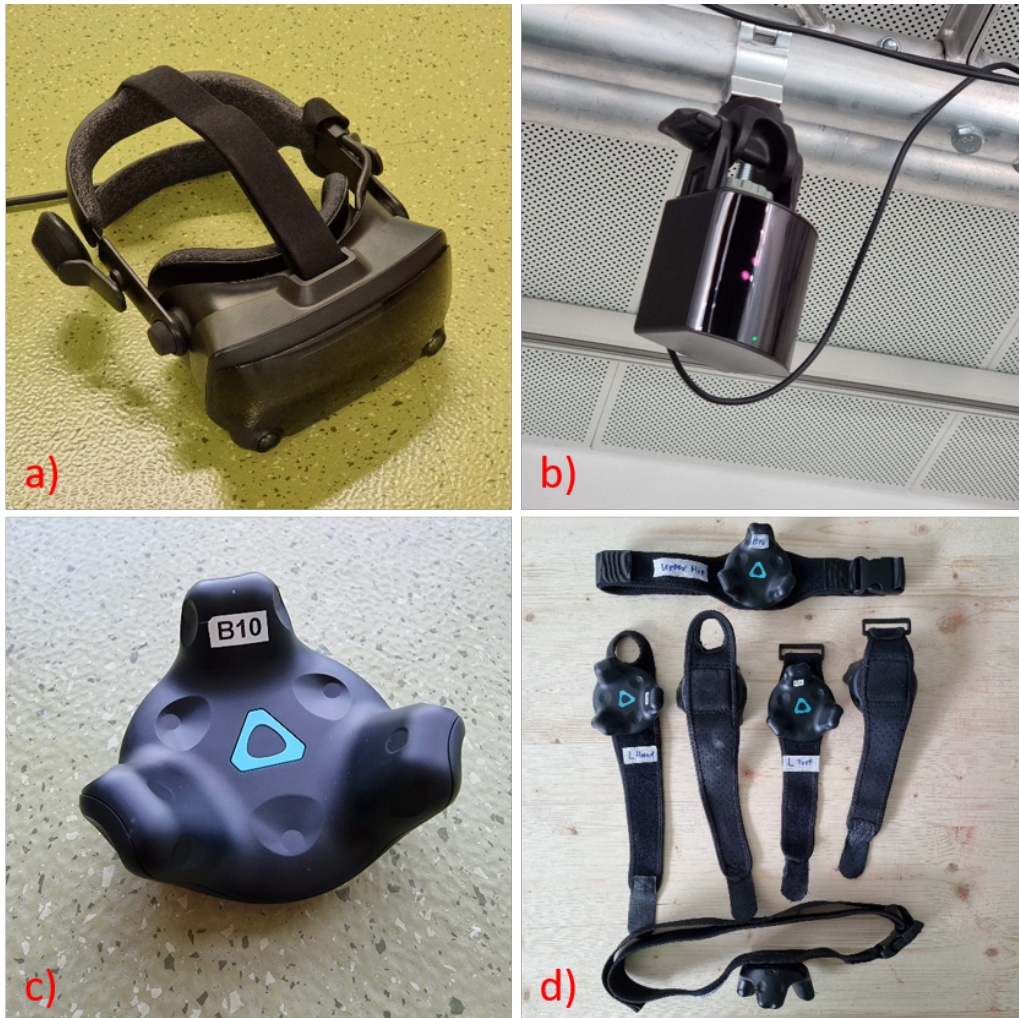
Figure 4.1.: Hardware utilised by E(x|g)o. a) Valve Index, b) base station, c) Vive Tracker 2, d) Vive Tracker 2 attached to Vive Tracker straps.
