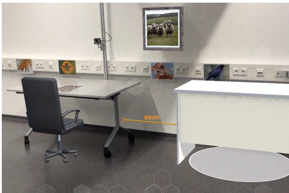
Figure 4.6.: HomePlanAR smart dynamic guides appearing between two aligned virtual and physical tables.
