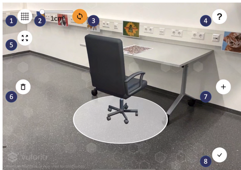
Figure 4.3.: HomePlanAR UI. (1) Switch to or deactivate grid; (2) scale grid; (3) align grid with selection or reset to default position; (4) open current study task; (5) switch to or deactivate smart dynamic guides; (6) delete selection; (7) open catalog; (8) confirm study task completion.
