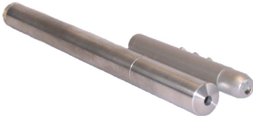
Figure 20: Version 1 of the interactive laser pointer based on a pen metaphor (built in December 2006). The laser pointer is equipped with a low power infrared laser diode, battery compartment, and an augmented button module with infrared transmission component (on top).
