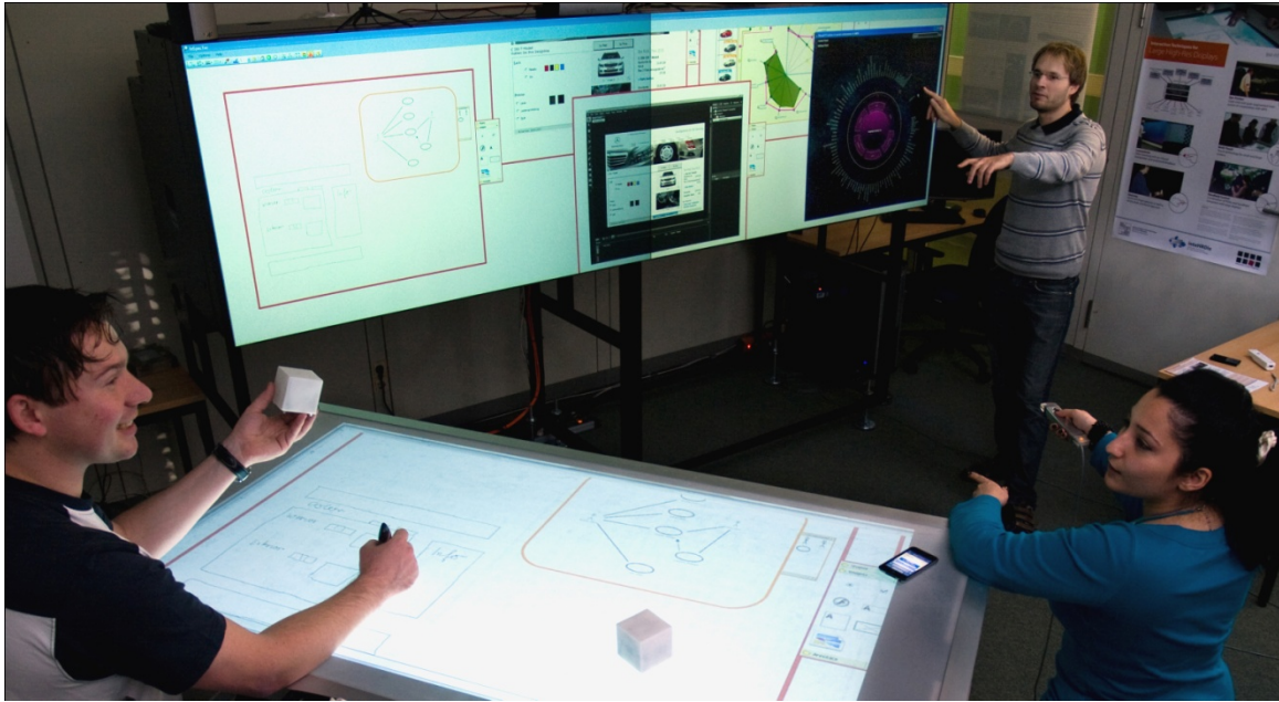
Figure 78: The Media Room is a lab environment which provides a variety of input and output devices with different modalities and form factors. Squidy serves as the basic technology for integrating these different devices as well as for configuring and evaluating them. http://hci.uni-konstanz.de/mediaroom
