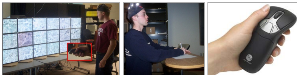
Figure 5: Participant using the wireless Gyration mouse with the 8x3 tiled LCD panel (left); the hat used to track participants' position (centre) [Ball et al. 2007]. Wireless Gyration 7 mouse (right).
