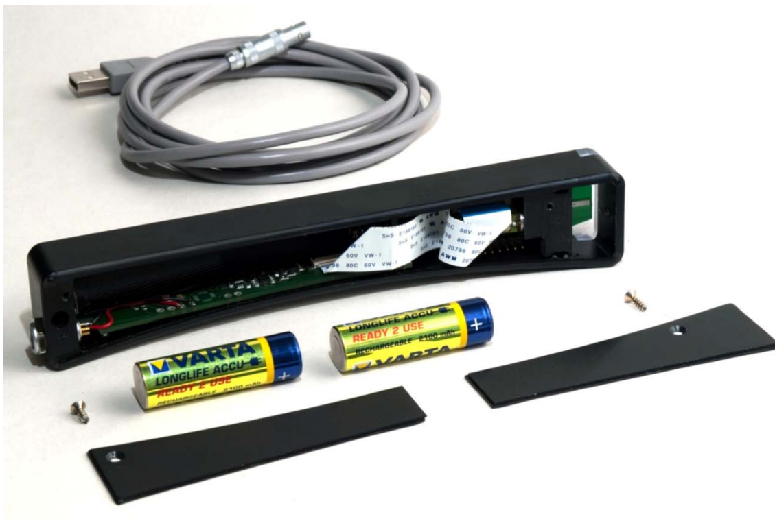
Figure 32: Interactive laser pointer with open battery compartment, released maintenance cover, rechargeable batteries, and USB charging cable. The covers can be slid in from the corresponding side (head or tail) and fixed with the screw. Thus the plain covers accommodate their form to the arched shape of the main case.
