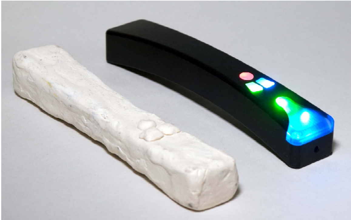
Figure 28: Initial clay model of the laser pointer (left) and the final device (right, built in October 2009).
