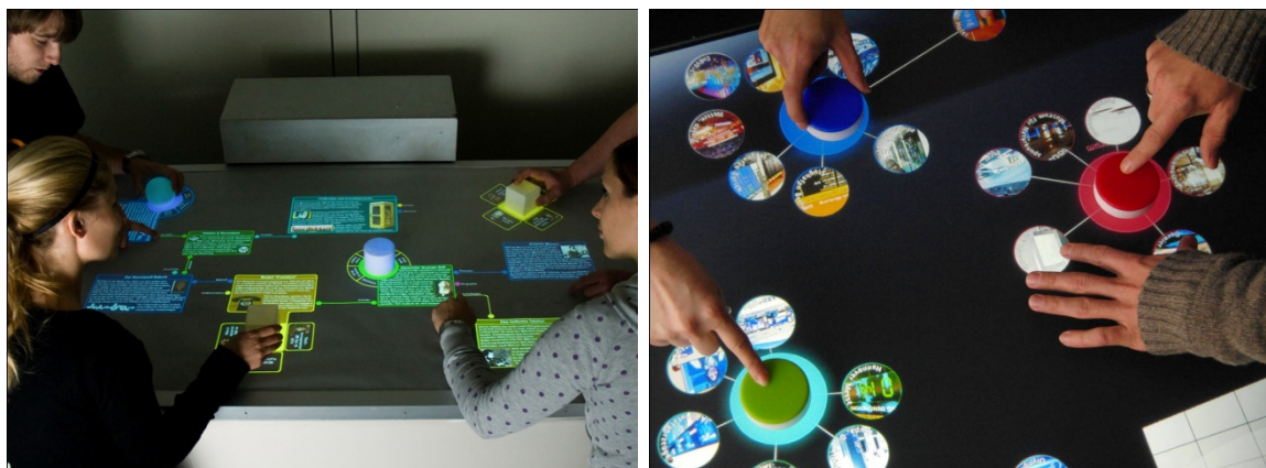
Figure 73: Multi-touch surfaces augmented with physical tokens used in the context of blended museum [Klinkhammer 2009] (left) and for interactive portfolio presentation of the ICT AG, Kohlberg 60 (right).
