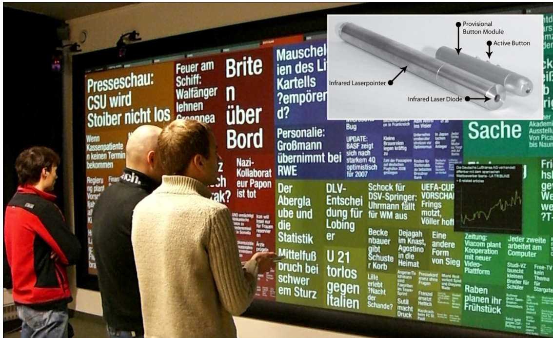
Figure 17: Newsmap visualization 14 on the Powerwall at the University of Konstanz controlled with the first version of our interactive laser pointer [König, Bieg & Reiterer 2007].
