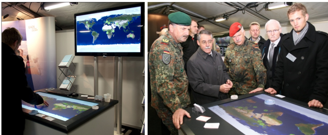
Figure 75: Research prototype illustrating the military help-desk workplace of the future – a multi-user and multi-display environment with multi-touch and token interaction. This prototype was developed as part of a close cooperation between EADS Defence & Security, Friedrichshafen, and the Human-Computer Interaction Group at the University of Konstanz. It was exhibited at the Symposium " Heereslogistik der Zukunft " organized by the German Army in Aachen, December 2009.
