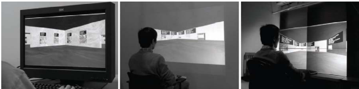
Figure 6: Display variants to evaluate individual and combined effects of display size and resolution on task performance: IBM T221 LCD as small display with high and alternatively low resolution (left). Rear-projection screen as large, low-resolution display (centre). VisBlocks: projection-based large, high-resolution display (right) [Ni et al. 2006].
