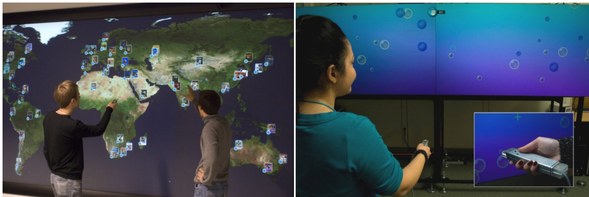
Figure 18: Laser pointer interaction at the large, high-resolution Powerwall of the University of Konstanz (left) and at the Cube Wall at the Media Room (right) consisting of two individual rear-projection displays each equipped with an infrared sensitive camera for optical tracking.
