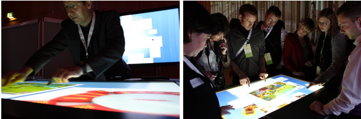
Figure 74: Creativity enhancing collaborative system based on multi-touch table, token interaction, digital pens, and peripheral wall display. The system was used as a moderation and presentation environment (left) and as a collaborative work environment (right) in the course of the workshop Creativity Think Tank 66 at the Creativity World Forum 2009 in Ludwigsburg. The multi-touch table and the token interaction were driven by the Squidy Interaction Library.
