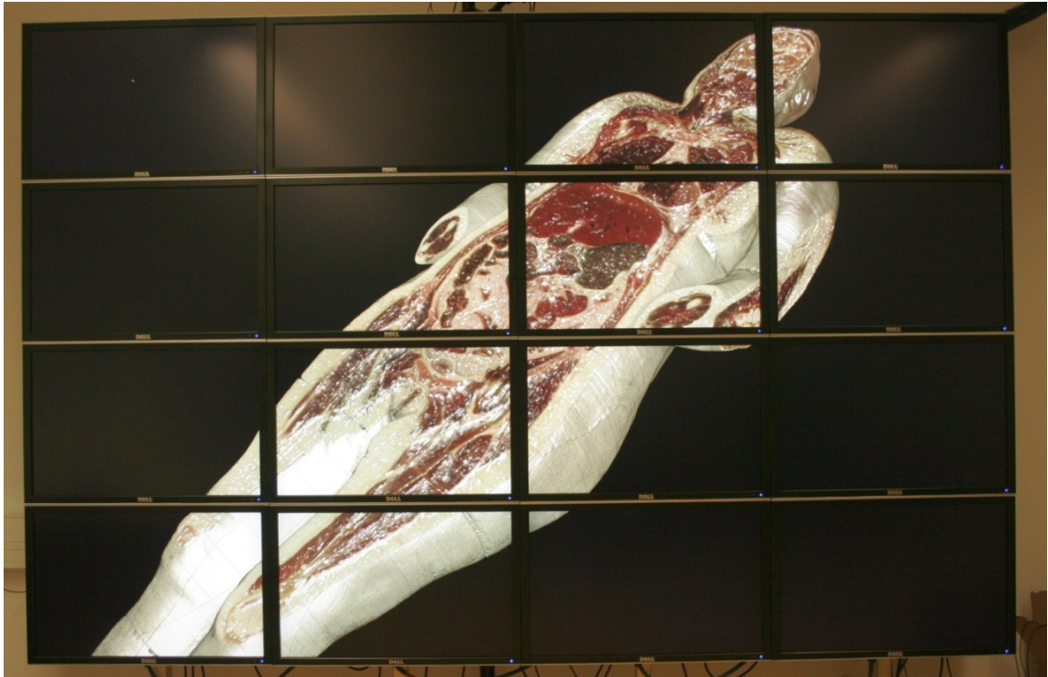
Figure 2: The „Visible Human Female“ data set is rendered in high-resolution on the GRIS Display Wall in Tübingen with a resolution of 10240 x 6400 pixels and a size of 2.8 x 2 meters. The wall consists of 4x4 30-inch LCDs and is powered by a cluster of 16 high-performance computers [Parys & Knittel 2009].
