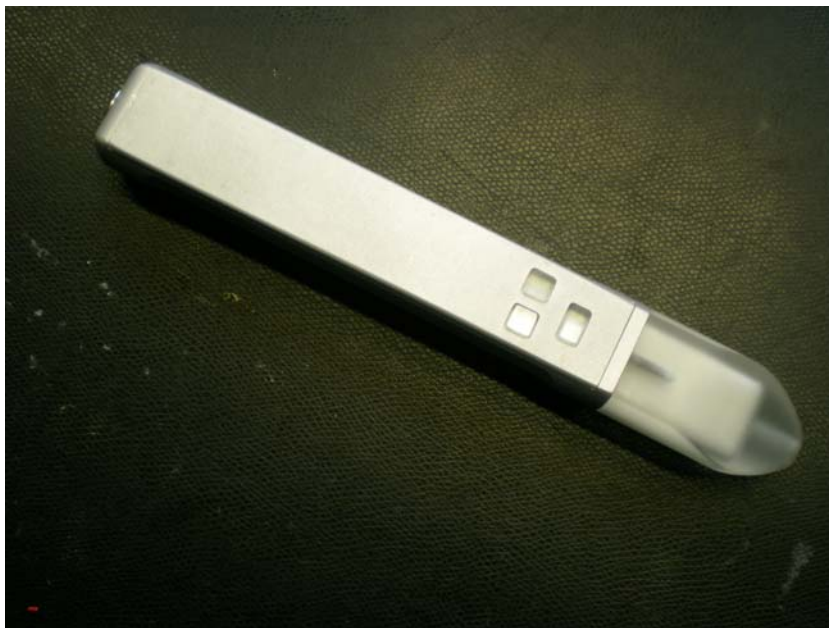
Figure 23: Prototype of the next laser pointer generation 3.5 (built in December 2008). The antenna is integrated within the translucent head and the lower side is rounded for better ergonomic handling. Since the hardware design was not satisfactory, development was not finished.
