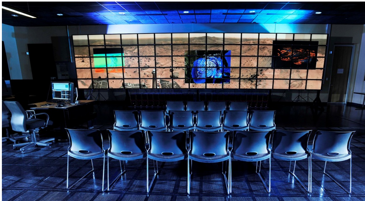
Figure 8: Stallion Cluster at the University of Texas: Ultra high-resolution display with 15x5 30 inch Dell LCD monitors and an overall resolution of 307 megapixels 9 .
