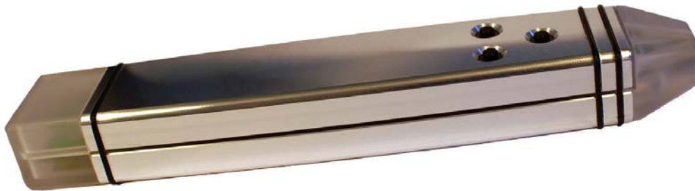
Figure 22: Version 3 of the interactive laser pointer with improved button module, visual feedback on both ends, accelerometer for gesture recognition, mechanical vibrator for tactile feedback, ZigBee wireless communication, and an alternative wired option (built in September 2007).
