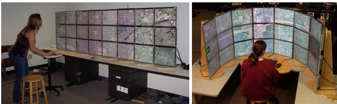
Figure 4: Tiled LCD panel with 24 monitors as flat (left) and as curved (right) wall display [Shupp et al. 2006].
