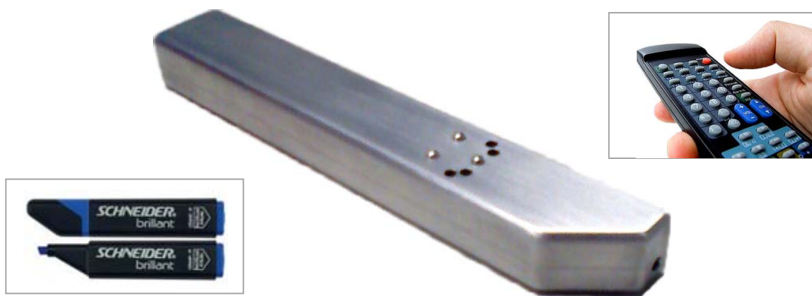
Figure 21: Second generation of our interactive laser pointer with embedded button module, multicolour LEDs for visual feedback and wireless communication based on ZigBee (built in June 2007). The case design supports two different handling styles: pen-like writing as known from text markers or controlling from distant positions as known from TV remote controls.
