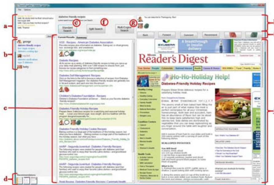
Figure 10 The SearchTogether Client (a) Integrating messaging, (b) query awareness, (c) current results, (d) recommendation queue, (e-g) search buttons, (h) page-specific metadata, (i) toolbar, (j) browser (Morris & Horvitz 2007)
