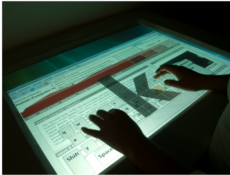
Figure 5.19: The user has just hit the letter “k”. This letter is displayed over the keyboard for a short duration and then faded out.
