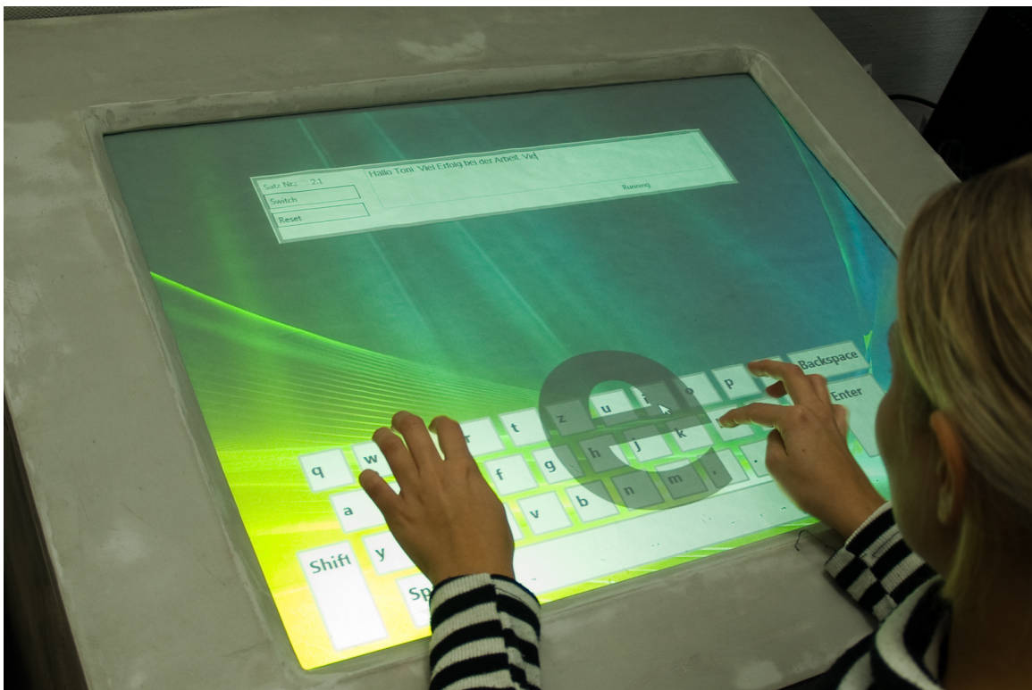
Figure 5.22: The user test setup. In this picture the participant enters a phrase using the Qwerty soft keyboard. The letter “e” indicates that she just hit the corresponding key. The text is entered into the white TextBox.
