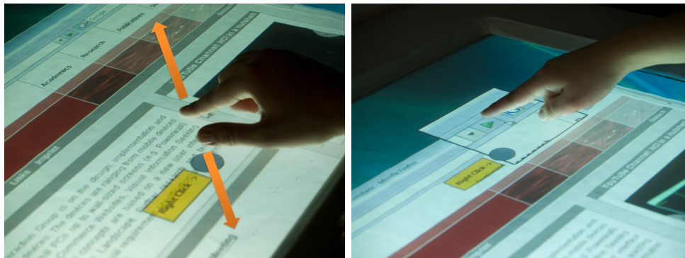
Figure 5.9: Left: ZoomTap’s local zoom is triggered by moving two fingers into different directions.
